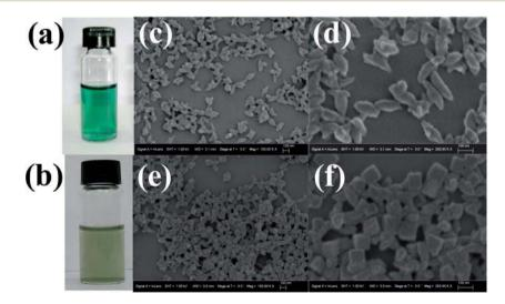
Fig. 1 Photographs of (a) PANI-PEC and (b) Ag@PANI-PEC dispersion in water; FE-SEM images of PANI-PEC (c and d) and Ag@PANI-PEC (e and f).
