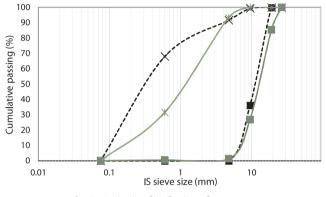
Fig. 2. Grain size distribution of aggregates.
