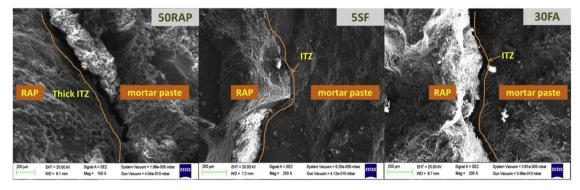
Fig. 5. Fe-SEM images showing ITZ of stated RAP-RCCP mixes.
