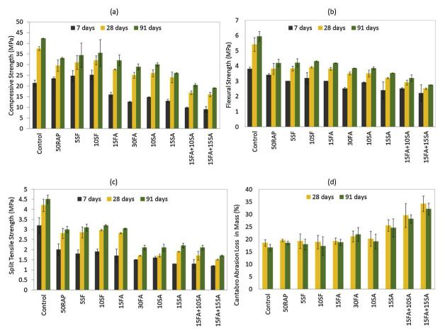
Fig. 4. (a) Compressive Strength, (b) Flexural Strength, (c) Split Tensile Strength, and (d) Cantabro Abrasion Loss.
