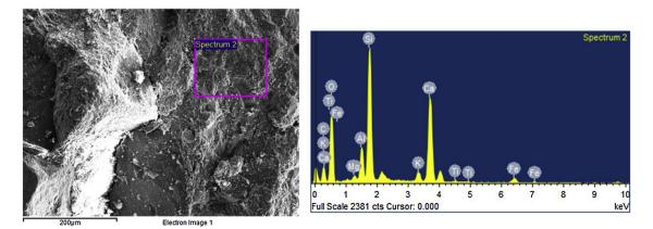
Fig. 11. EDX pattern of 50RAP mix containing 5% silica fume.
