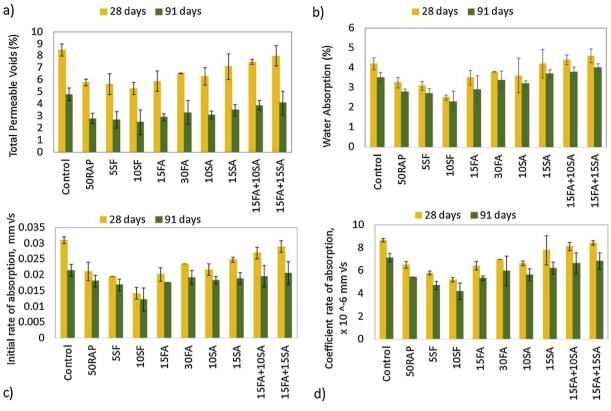
Fig. 8. (a) Porosity, (b) water absorption, (c) initial rate of absorption, and (d) coefficient rate of absorption.
