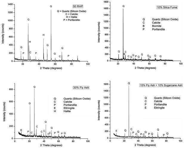
Fig. 6. XRD patterns of stated RAP-RCCP mixes.
