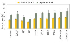
Fig. 12. Effect of SCMs after exposure to acid attack.
