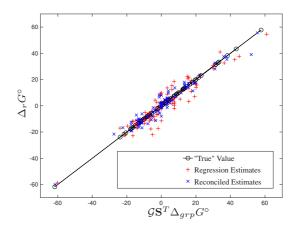
Fig. 4. Results of the modified group contribution showing that the reconciled estimates are more thermodynamically consistent (constraint error of 3.77 kJ/mol) than the regression estimates (constraint error of 5.83 kJ/mol). Morever, the reconciled estimates of group contributions yield reaction energies that are closer to the "true" values. (RMSE of 5.35 kJ/mol compared to 6.05 kJ/mol for the Pseudoisomer group contribution (PGC)
