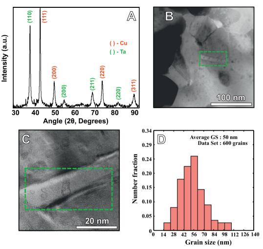
Fig. 1. (A) XRD peaks for as-received NC Cu-Ta alloy. (B) BFSTEM image of as-received NC Cu-Ta alloy microstructure. (C) As-received HRTEM image of NC Cu-Ta alloy highlighting the segregation of Ta nano-clusters within the microstructure. (D) As received, grain size distribution for Cu.
