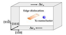
**Fig. A1.** Schematic of the simulation setup showing an edge dislocation and a Ta nanocluster in a single Cu nanocrystal where X, Y and Z correspond to  $[1\overline{10}]$ ,  $[11\overline{2}]$  and [111] directions respectively.
