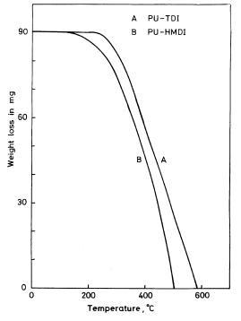
Figure 2. Thermal stabilities of polyurethanes.
