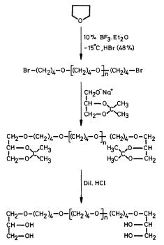
Scheme 1. Schematic representation of preparing tetrahydroxyl-terminated polytetrahydrofuran.
