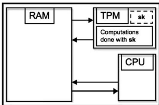
**Figure 1.** A hybrid system with trusted platform module deployed.
