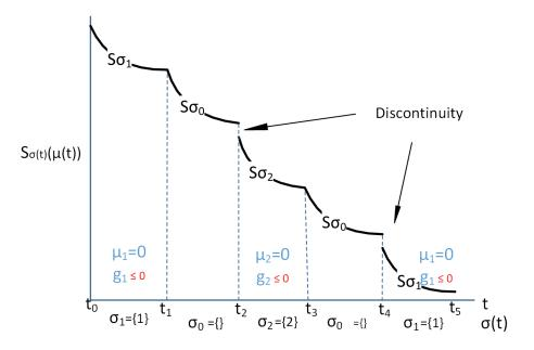
Figure 8: Example for time evolution of storage function with two inequality constraints (p = 2). Note that case (i) appears at switching time  $t_2$ ,  $t_4$  and case (ii) at  $t_1$ ,  $t_3$ .
