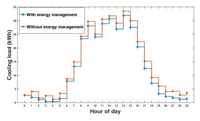
Figure 7: Cooling load
