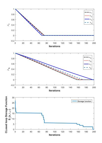
Figure 3: The case study in Section 5 have four zones, each zone temperature has an upper and lower bound, giving rise to eight inequality constraints. When an inequality constraint is feasible (i.e.  $g_i(T) \leq 0$  see Fig. 4) and its corresponding Lagrange variable ( $\mu_i$ ) converge to zero, then the closed loop storage function switches to a new storage function that is strictly less than the current one, causing a discontinuity.
