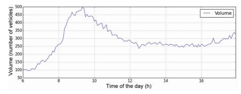
Figure 6. Flow (at 5 min intervals) for different hours of the day.
