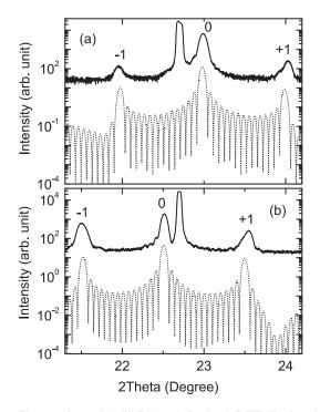
FIG. 1. The experimental (solid line) and simulated (DIFFaX) (dotted line)  $\theta$ -2 $\theta$  x-ray diffraction profiles of (a) (001)STO/[20-u.c. LSMO/3-u.c. SRO]<sub>x15</sub> and (b) (001)STO/[20-u.c. SRO/3-u.c. LSMO]<sub>x15</sub> superlattices. The (001) Bragg's reflection of STO as well as the satellite peaks (0th and ± 1st orders) are indicated.
