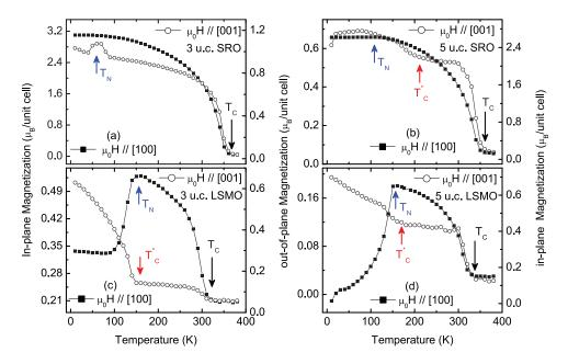
FIG. 2. (Color online) Temperature dependent 0.1 tesla field cooled magnetization of (a) (001)STO/[20-u.c. LSMO/3-u.c. SRO]<sub>x15</sub>, (b) (001)STO/[20-u.c. LSMO/5-u.c. SRO]<sub>x15</sub>, (c) (001)STO/[20-u.c. SRO/3-u.c. LSMO]<sub>x15</sub>, and (d) (001)STO/ [20-u.c. SRO/5-u.c. LSMO]<sub>x15</sub> superlattices with field oriented along the plane and out-of-plane. The arrows indicate the  $T_C$ ,  $T_C^*$ , and  $T_N$ .
