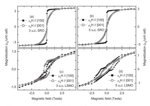
FIG. 3. Field dependent magnetization at 10 K with field oriented along the plane and out-of-plane of (a) (001)STO/[20-u.c. LSMO/3-u.c. SRO]\_{x15}, (b) (001)STO/[20-u.c. LSMO/5-u.c. SRO]\_{x15}, (c) (001)STO/[20-u.c. SRO/3-u.c. LSMO]\_{x15}, and (d) (001)STO/[20-u.c. SRO/5-u.c. LSMO]\_{x15} superlattices.
