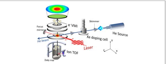
**Figure 1.** Schematic illustration of the experimental setup. The He droplet source, doping cell and spectrometer are contained in differentially-pumped vacuum chambers separated by beam skimmers. Electrons are imaged on an imaging detector at the top of the spectrometer; ions are detected by a Daly type TOF detector at the bottom. The laser beam is back focused into the He droplet beam at right angles by a spherical mirror (f = 75 mm).
