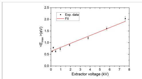
Figure 10. Dependence of the mean electron peak energy on the extractor voltage for  $He_{8000}Xe_{12}$  irradiated by NIR pulses. The red line is a linear fit of the data.
