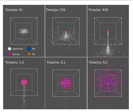
**Figure 11.** Theoretical time-evolution of a nanoplasma ignited by an intense NIR laser pulse in the presence of an external homogeneous electric field ( $F = 1000 \text{ V cm}^{-1}$ ). The laser polarization is horizontal and the electric field points upwards.
