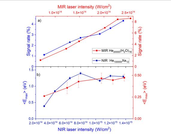
**Figure 7.** Laser intensity dependence. (a) Nanoplasma hit rate for He droplets irradiated by NIR and MIR pulses at different intensities. (b) Electron peak energy for the two laser types. Notice that the blue axis (bottom and left) corresponds to the NIR data and the red (top and right) to the MIR data.
