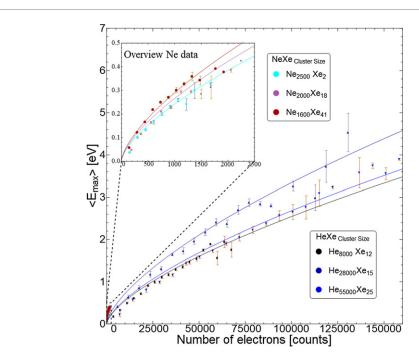
**Figure 9.** Peak electron energies as a function of the number of nanoplasma electrons. The data points represent the mean values of the distributions of electron peak energies for different He and Ne cluster sizes. The solid lines represent the fits based on equation (3). The inset shows a closeup of the low-energy region where the Ne data points are concentrated.
