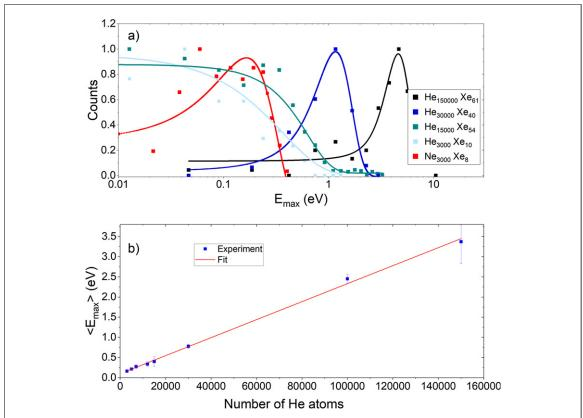
**Figure 5.** (a) Histograms of the electron peak energies  $E_{\text{max}}$  of the single-shot VMIs that were averaged in figure 4. The data points are the energies for the different He and Ne clusters sizes. The solid lines are Gaussian fits. (b) Cluster size dependence of the mean peak energy for the He data shown in (a) including additional cluster sizes. The red line is a linear fit of the experimental data.
