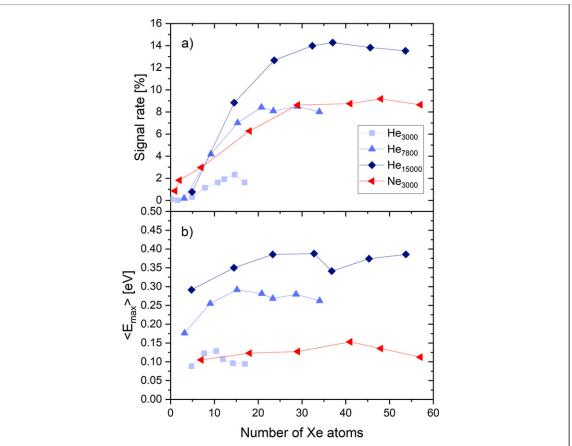
**Figure 6.** Dependence on the number of dopant atoms. (a) Fraction of VMIs containing nanoplasma electrons for different He and Ne cluster sizes ionized by NIR pulse. (b) Mean electron peak energy. The blue symbols correspond to He droplets of different sizes, the red symbols correspond to Ne<sub>3000</sub>.
