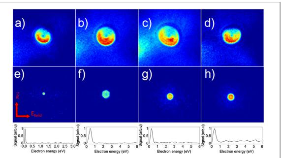
Figure 3. Selected single-shot electron images of Ne clusters. (a)–(d) Large Ne clusters consisting of on average 6000 Ne atoms doped with 10 Xe atoms ionized by an MIR laser pulses. (e)–(h)  $Ne_{2000}Xe_8$  and their respective electron spectra (bottom row) ionized by NIR pulses.
