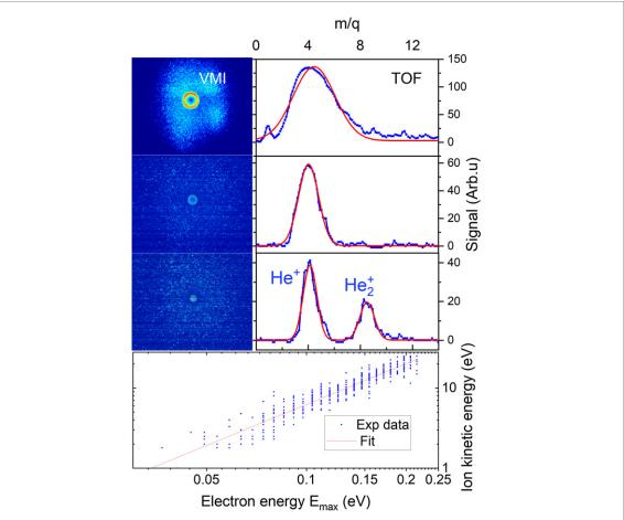
**Figure 8.** Selected single-shot electron VMIs of He droplets of size 10<sup>4</sup> He atoms doped with calcium atoms, irradiated by MIR pulses, and ion TOF mass-over-charge spectra measured simultaneously. Blue lines are the experimental data, red lines are Gaussian fits. The bottom panel represents ion kinetic energies inferred from the fits vs electron peak energies for individual correlated single-shot electron VMIs and ion TOF traces. The red line is a power-law fit.
