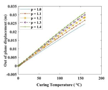
Figure 5: Out of plane displacement with curing temperature for L=150 mm
