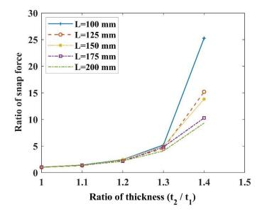
Figure 7: Ratio of snap forces with thickness variation
