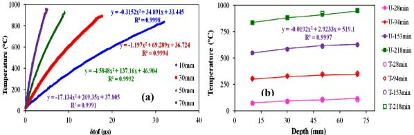
Fig.2. (a) The  $\delta$ TOF vs. Temperature obtained from multiple sensor of helical waveguide; (b) The ultrasonic temperature measurements vs different depths at different time instances during a heating cycle inside a furnace. Here, U represents ultrasonic measurements and T represents corresponding thermocouple readings.
