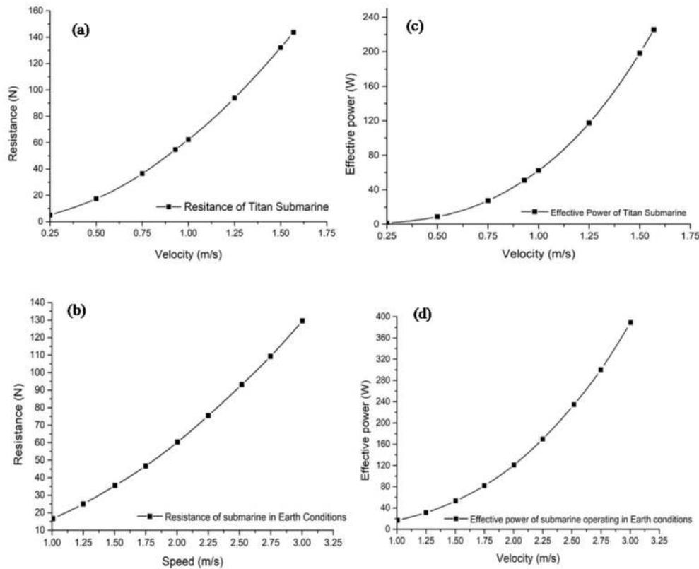
Fig. 20. (a, b) Resistance and (c, d) effective power of submarine operating in Titan’s and Earth’s environments [98].
