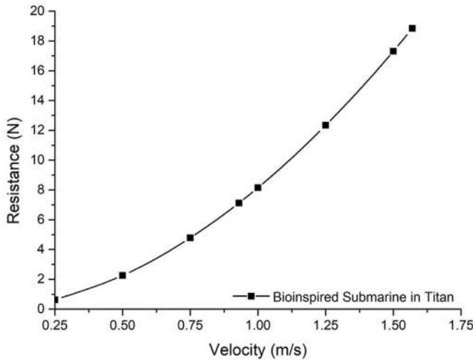
Fig. 21. Resistance of bio-inspired submarine operating in Titan environment [98].
