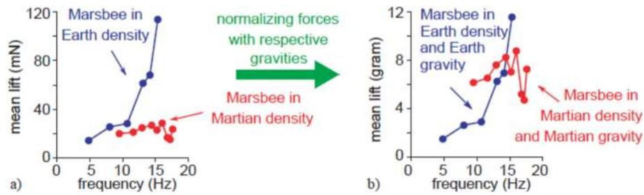
Fig. 9. Lift force generation of a Marsbee in (a) Earth and (b) simulated Martian atmospheric conditions [15].
