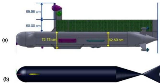
Fig. 11. (a) Conventional Titan submarine fitted with thrusters [98]. (b) Proposed bio-inspired AUV for Titan [99].
