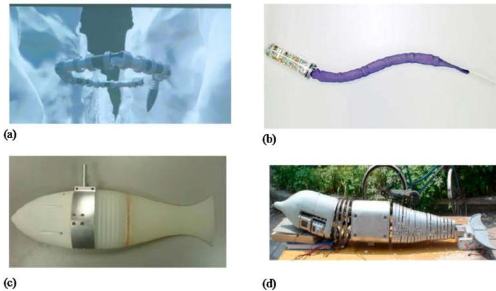
Fig. 4. Bioinspired underwater vehicles. (a) EEL fish robot [45], (b) Lamprey robot [46]), (c) Trout robot [115], and (d) Dolphin robot [47].
