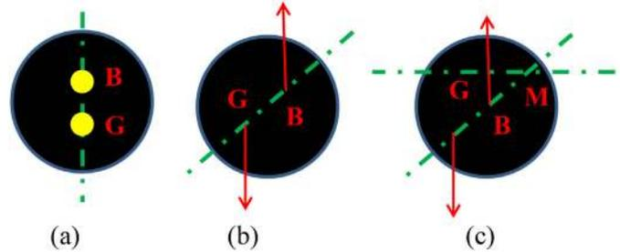
Fig. 15. (a) Submerged vehicle in transversely stable equilibrium, (b) small heel when B is above G, and (c) heel angle floating on the surface.
