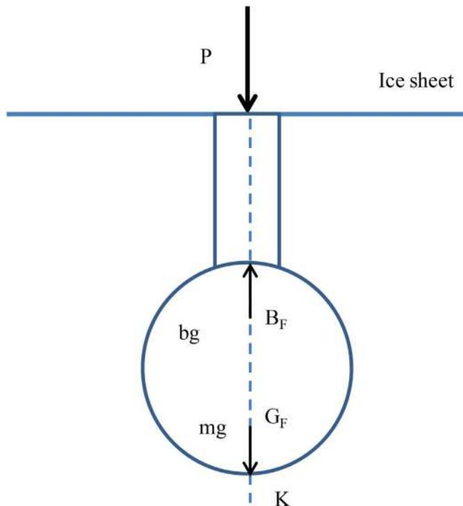
Fig. 18. Underwater vehicle breaking through ice [100].
