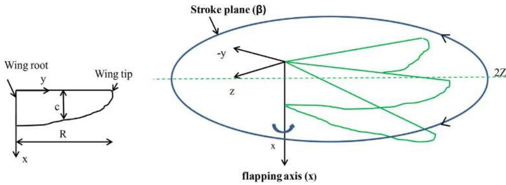
Fig. 7. (a) Schematic illustration of semi-elliptic insect flapping wing, and (b) flapping motion.
