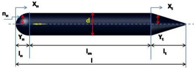
Fig. 13. Geometry of hull form.
