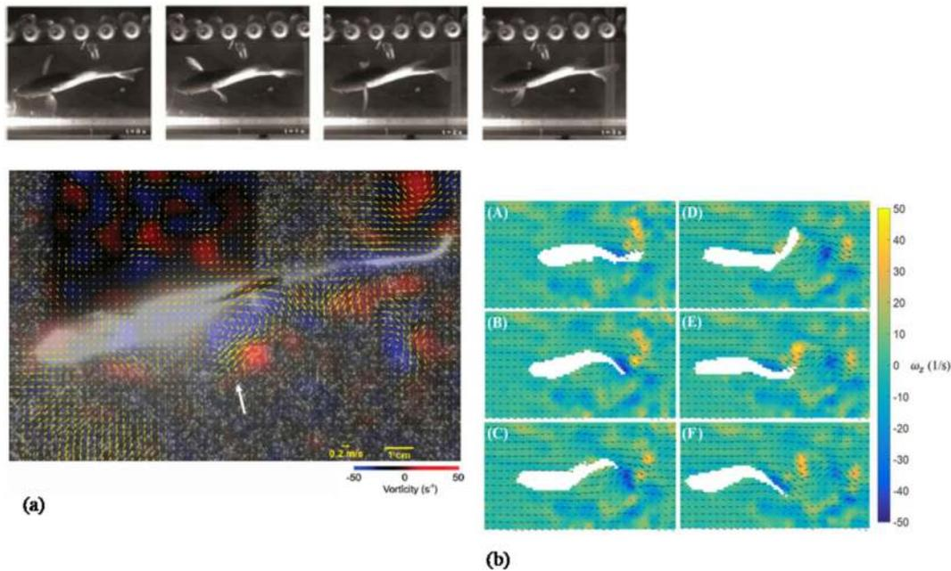
Fig. 5. (a) PIV analysis of bluegill sunfish swimming backwards raw image (top row) and Anal fin vortices (second row) [57]. (b) Zebrafish swimming in cruising mode [58].
