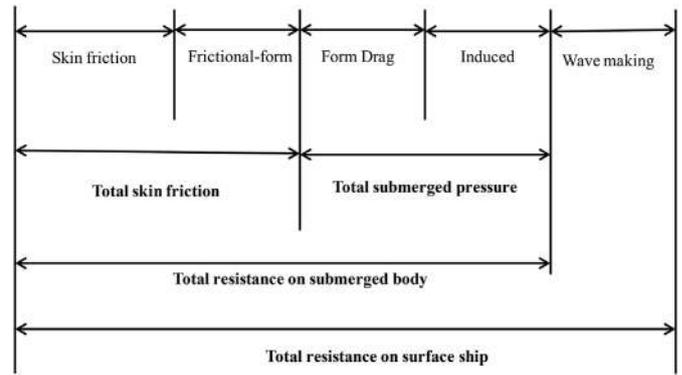
Fig. 19. Components of resistance for submerged body.
