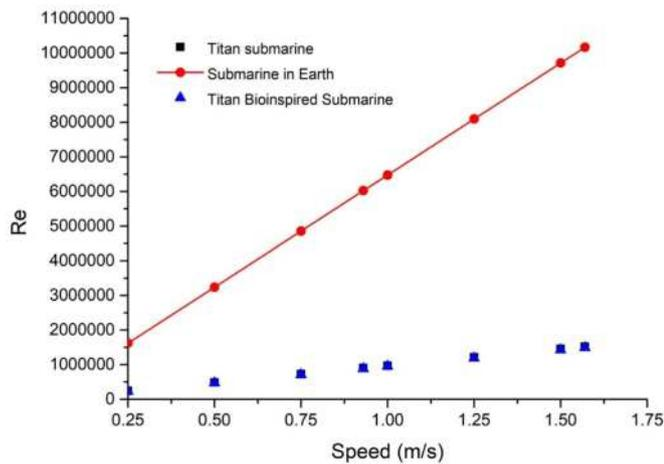
Fig. 23. Effect of speed on Reynolds number in Titan and Earth conditions [98].
