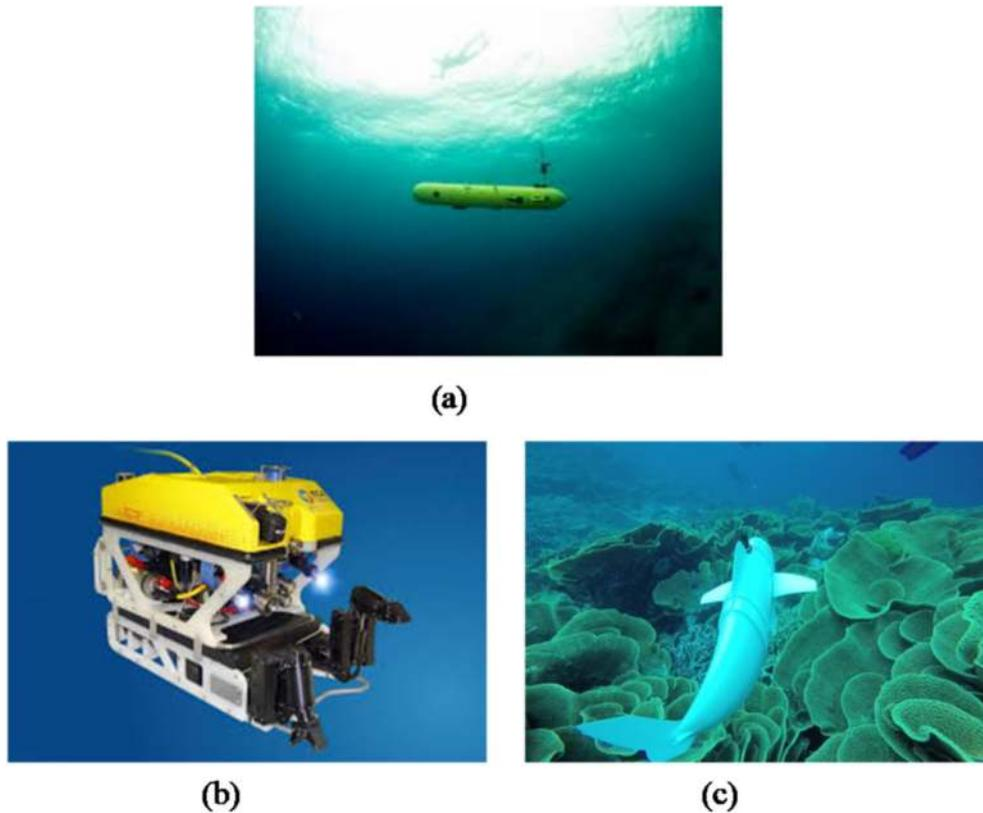
Fig. 1. Types of underwater vehicles. (a) autonomous underwater vehicle, (b) remotely operated vehicle, and (c) biomimetic underwater vehicle [108].
