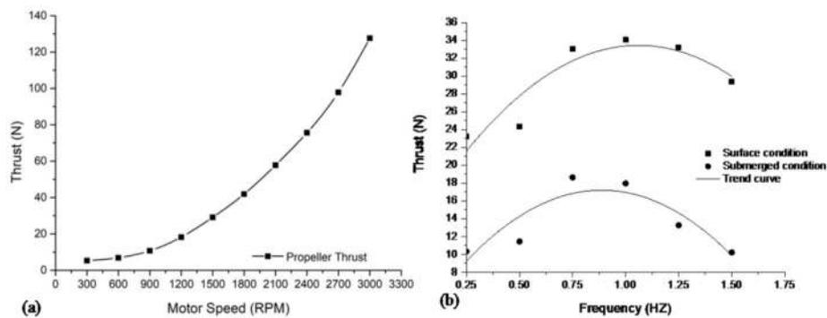
Fig. 22. (a) Thrust performance of propeller operating in Titan environment [107]. (b) Thrust performance of bioinspired submarine in Earth's environment [108].
