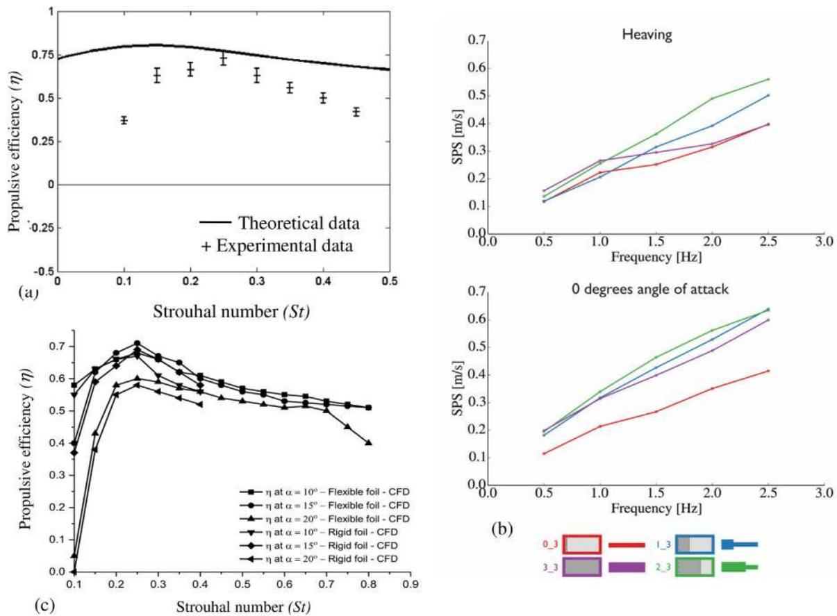
Fig. 3. (a) Propulsive efficiency ( $\eta$ ) of flapping foil as a function of Strouhal number ( $St$ ) [35]. (b) Self-propelled speeds (SPS) of swimming foils (0\_3 – single layer low stiffness material, 3\_3 – triple layer high stiffness material, 1\_3 and 2\_3 – the anterior 1/3 and 2/3 of foil contains high stiffened material) [36]. (c) Propulsive efficiency of flapping foil [37].
