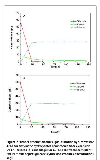
xylose remained unused even after 72 h (Figure 7). Ethanol concentration in the broth was 28 g/L after 72 h, which corresponds to 93% theoretical yield based on total sugar consumption. In untreated silage, 23 g/L ethanol with a metabolic yield of 98% was produced at 72 h (data not shown).
