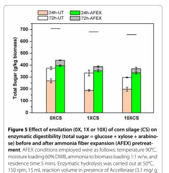
of cellulose) and Stargen (3.8 mg/g of starch). The lines above all bars indicate the maximum possible total sugar yield based on theoretical composition. matic digestibility of cellulose by cleaving LCC linkages [24]. The mechanisms by which lignin restricts cell wall degradation and hydrolysis of cellulose are not well understood. Enteric fermentation studies suggest that the influence of lignin on microbial deconstruction of plant cell walls may be primarily due to physical mechanisms
