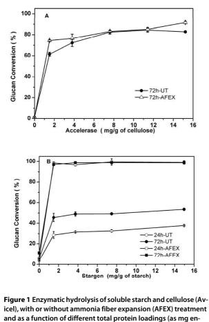
zyme/gram glucan). Cellulose and starch hydrolysis carried out using (a) Accellerase and (b) Stargen.
