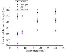
**Fig. 4** Laser energy versus diameter of micro-dimple for different ambient conditions (Energy 5, 8, 18, 30 mJ, No of pulses=100).
