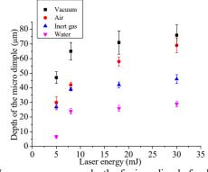
Fig. 7 Laser energy versus depth of micro-dimple for different ambient conditions (Energy 5, 8, 18, 30 mJ, No of pulses=100).
