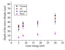
Fig. 6 Laser energy versus depth of micro-dimple for different ambient conditions (Energy 5, 8, 18, 30 mJ, No of pulses=50).
