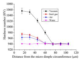
**Fig. 14** Measurement of Vickers hardness as a function of radial distance from the micro-dimple circumference for different ambient conditions (Energy 5 mJ and 50 pulses).
