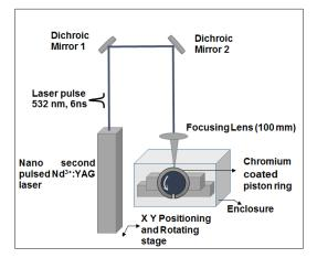
Fig. 1 Experimental set up.
