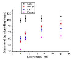
Fig. 3 Laser energy versus diameter of micro-dimple for different ambient conditions (Energy 5, 8, 18, 30 mJ, No of pulses=50).
