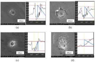
**Fig. 10** SEM images and the corresponding depth profile of the micro-dimple made in (a) Air, (b) Inert gas (Ar), (c) Vacuum and (d) Water. All micro-dimples were formed with 5 mJ and 50 pulses.
