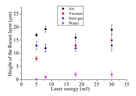
Fig. 8 Height of the recast layer bulges as a function of laser energy for different ambient conditions, No of pulses=50.
