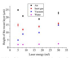
Fig. 9 Height of the recast layer around the micro-dimple as a function of laser energy for different ambient conditions, No of pulses=100.
