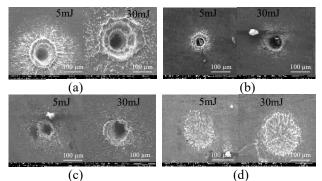
**Fig. 5** Variation of micro-dimple dimension for 100 pulses (a) Air, (b) Vacuum, (c) Inert gas (Ar) and (d) Water.
