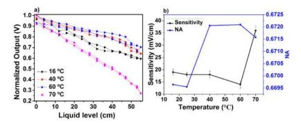
**Fig. 4.** (a) The relationship between normalized voltage and the liquid level with temperature various of 16 °C, 40 °C, 60 °C and 70 °C (b) The relationship between sensitivity vs temperature of 16 °C, 25 °C, 40 °C, 60 °C and 70 °C (b) The relationship between sensitivity of 1.9, 1.8, 1.4, and 3.6 mV/mm respectively.
