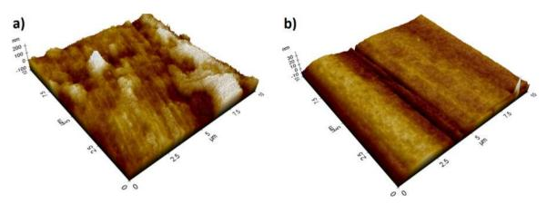
Fig. 6. AFM of a) decladded POF b) bare POF. Decladded POF shows a rough surface through the decladded surface with a roughness of 80 nm whereas the bare POF shows a smooth surface over the entire length.
