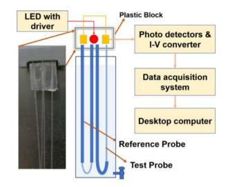
**Fig. 1.** Schematic showing block diagram of experimental setup consists of two Ubent POFs (decladded region of fiber represented as a thin line) dipped in a 55 cm long liquid column, home-made plastic block to house LED and PDs, optoelectronic circuitry, and DAQ.
