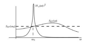
Fig. 2: Equivalent white noise excitation (Image courtesy: Lutes and Sarkani [3]).
