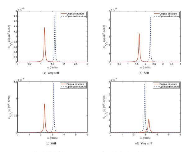
Fig. 4: PSDF of the response at top storey for original and optimized structure.
