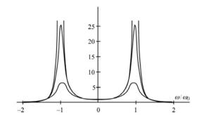
Fig. 1: Plot of  $|H(\omega)|^2$  for  $\xi = 0.05, 0.10, 0.20$  (Image courtesy: Lutes and Sarkani [3]).
