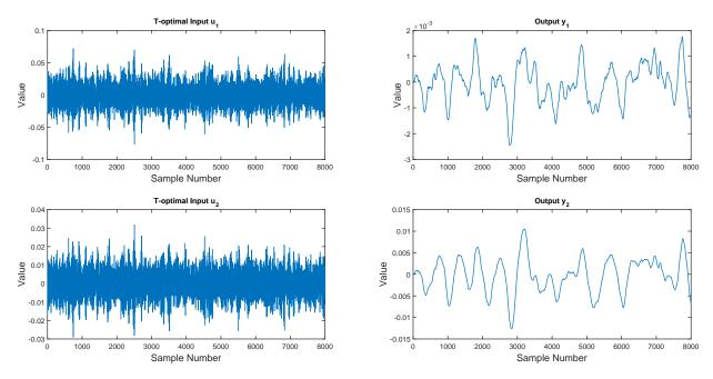
Figure 8: The inputs corresponding to the  $\mathcal{T}$ -optimal spectrum are shown on the left. The outputs obtained by exciting the system with the inputs are shown to the right.
