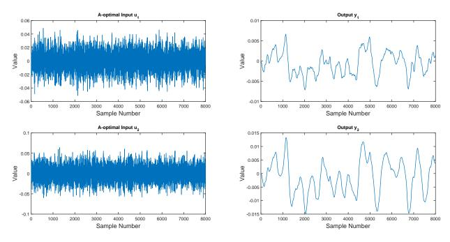
Figure 7: The inputs corresponding to the  $\mathcal{A}$ -optimal spectrum are shown on the left. The outputs obtained by exciting the system with the inputs are shown to the right.
