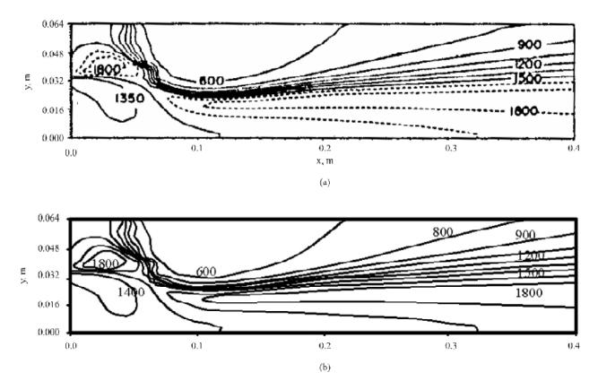
Figure 4. Temperature (K) contours: (a) Cherng<sup>1</sup>, et al. and (b) present study (numerical).
