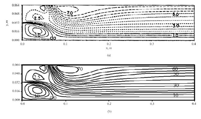
Figure 3. Streamline pattern: (a) Cherng<sup>1</sup>, et al. and (b) present study (numerical).
