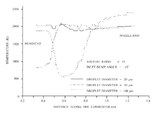
Figure 11. Effect of fuel droplet size on centreline variations of temperature.
