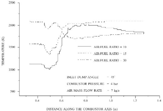
Figure 10. Effect of air/fuel ratio on centreline variations of temperature.
