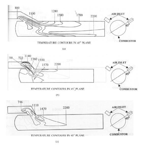
Figure 8. Temperature contours for different air-inlet dump angles: (a) 30°, (b) 45°, and (c) 60°.
