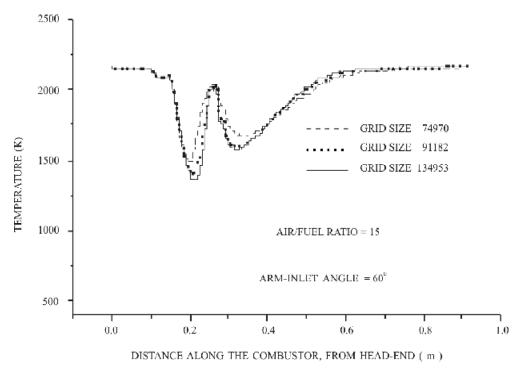
Figure 2. Static temperature variations along the combustor axis.
