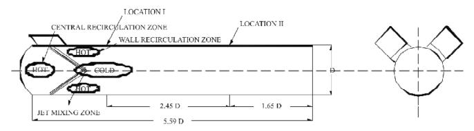
Figure 1. Ramjet dump combustor configuration used for simulation.
