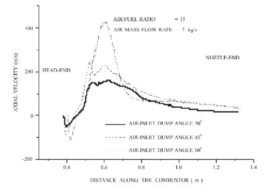
Figure 5. Effect of air-inlet dump angle on centreline value of u - velocity.
