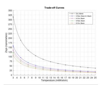
**FIG. 2.** Trade-off curves between  $T_{sys}$  and  $Z_{sys}$  for different geometries as discussed in Tables II and III.
