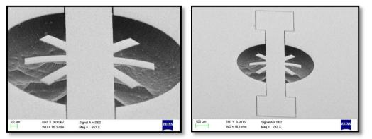
Figure 6: SEM images of the NiTi micro-wrapper and TiN micro-heater structures after bottom Silicon etch
