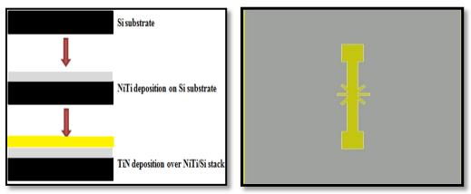
Figure 4: (a) Process flow of Si/NiTi/TiN stack (b) The CAD design of NiTi/TiN micro structures
