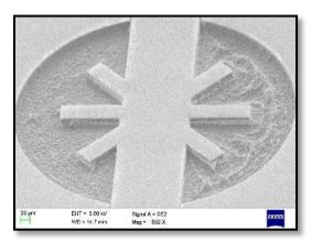
Figure 5: Femtosecond laser micro-machined NiTi micro-wrapper and TiN micro-heater structures
