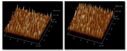
Figure 3: AFM 3D image of pulsed DC sputter deposited NiTi film (a) room temperature, (b) elevated temperature
