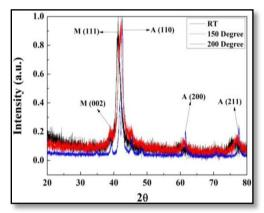
Figure 1: High temperature X-Ray diffraction spectra of pulsed DC sputter deposited NiTi films
