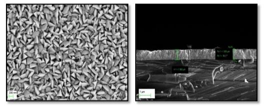
**Figure 2:** (a) Scanning electron microscopic image of the surface topography of pulsed DC sputter deposited NiTi thin films, (b) Fractured cross-sectional image of NiTi films
