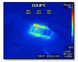
Figure 7: IR image of the temperature generated by TiN micro-heater
