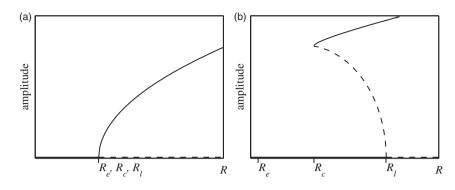
**Figure 1.** The steady state oscillation amplitude,  $a_{SS}$ , as a function of a control parameter, R, for (a) a supercritical bifurcation and (b) a subcritical bifurcation.  $R_I$  is the point at which the fixed point (i.e., the zero amplitude solution) becomes unstable.  $R_c$  is the point below which no oscillations can be sustained and  $R_e$  is the point below which all perturbations decrease monotically to zero.
