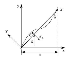
**Figure 21.** Geometry of an axi-symmetric wedge flame stabilized on a wire. Here  $\xi'$  is the displacement of instantaneous flame shape from the unperturbed flame shape along X,  $\alpha$  is the flame angle,  $S_L$  is the laminar flame speed, b is the radius of the burner, and  $\bar{u}$  is the mean flow. Figure reproduced with permission from Subramanian and Sujith.<sup>39</sup>
