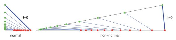
**Figure 3.** Geometric sketch of energy growth/decay in a two-dimensional orthogonal (left) and nonorthogonal (right) system. In either case, the two vector components contract, ultimately yielding a solution vector of zero length. In the normal case, monotonic decay toward a zero-length solution is observed; in the non-normal case, transient growth prevails before the asymptotic limit of a zero-length vector is reached.
