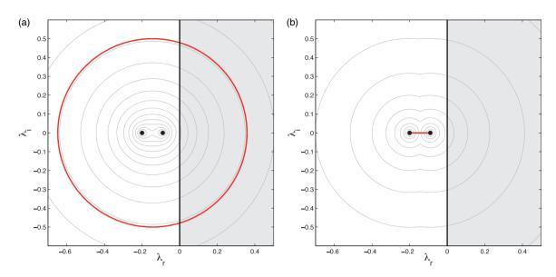
**Figure 4.** (a) Boundary of the numerical range (in red) and spectrum (in black symbols) of the non-normal matrix A for Re = 10. (b) Boundary of the numerical range (in red) and spectrum (in black symbols) of A when the off-diagonal term is set to zero, thus rendering A a normal matrix.
