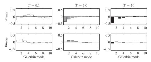
**Figure 19.** Initial states that give maximum transient growth at  $E_0 = 0.1099$  for T = 0.1, T = 1.0, and T = 10. The optimal initial state with T = 10 has most energy in the first mode and appreciable energy in the third and fourth modes.
