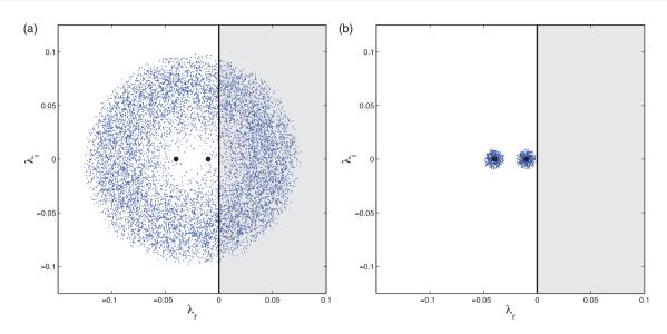
**Figure 6.** Sensitivity of eigenvalues for (a) the non-normal system at Re = 50, and (b) the normal system (with zero off-diagonal term) at the same Reynolds number. In both cases, the matrix A has been perturbed by random matrices of norm  $10^{-2}$ .
