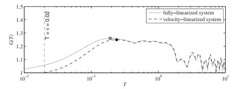
**Figure 12.** Maximum transient growth, G(T), as a function of optimization time, T, for the 10 mode Rijke tube with  $x_f = 0.3$ ,  $c_1 = 0.05$ ,  $c_2 = 0.01$ ,  $\tau = 0.02$ , and  $\beta = 0.75$  for the fully-linearized system (solid line). The maximum value is  $G_{max} = 1.26$  at T = 0.2.
