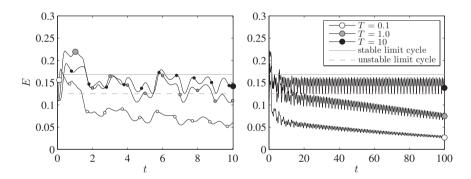
**Figure 20.** Energy, *E*, as a function of time, *t*, for the three initial states in Figure 19. The optimal initial state with T = 10 has smaller transient growth at short times but then grows to the stable limit cycle (not shown).
