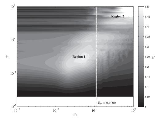
**Figure 17.** Transient growth,  $G(T,E_0)$ , as a function of optimization time, T and initial energy,  $E_0$ , for perturbations around the fixed point of the Rijke tube.
