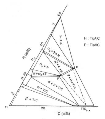
Fig.3 The phase diagram<sup>24)</sup> of Ti-Al-C ternary system at 1050°C.
