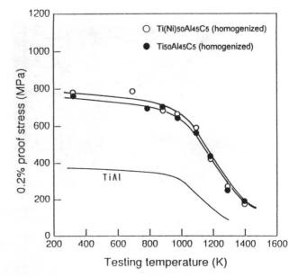
Fig.5 Compressive 0.2 % proof strength as a function of the testing temperature. Included for purpose of comparison is the proof strength of binary TiAl alloy.
