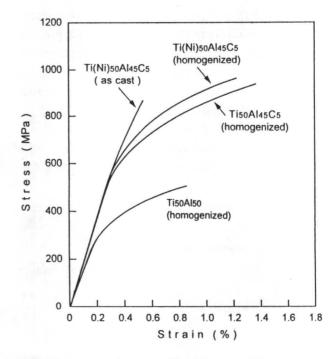
Fig.6 The stress-strain curves of bend tests at ambient temperature.
