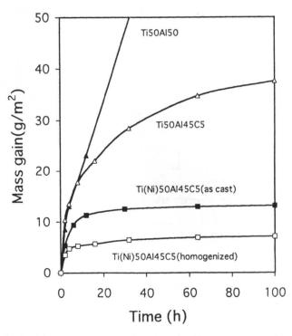
Fig.9 Mass gain curves as a function of oxidation time at 900°C in air.
