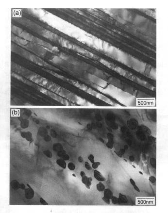
Fig.4 TEM micrographs of the composite with impurities (Ti(Ni)<sub>50</sub>Al<sub>45</sub>C<sub>5</sub>), showing smaller precipitates in place of lamellar disappeared; (a) as cast, and (b) homogenized at 1000°C.
