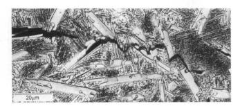
Fig.8 An optical micrograph taken at the crack tip of the composite with impurities (Ti(Ni)<sub>50</sub>Al<sub>45</sub>C<sub>5</sub>) homogenized at 1000°C.
