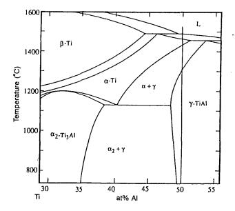
Fig.1 The central portion of binary Ti-Al equilibrium phase diagram<sup>23)</sup> showing estimated matrix composition and homogenizing temperature for the alloys used.
