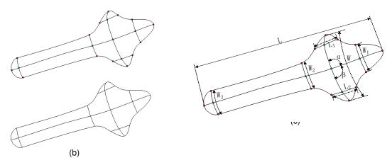
Figure 4: Parameterization of the abutted surface.
