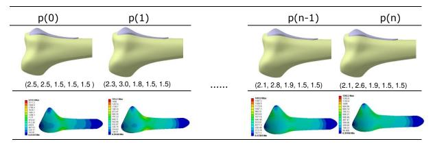
Figure 13: Optimizing the III type of plate by modifying thickness parameters.
