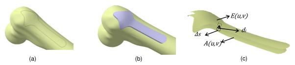
**Figure 9:** Volume of plate and its calculation: (a) Abutted surface, (b) Volumetric plate, (c) A represents abutted surface and E represents outside surface.
