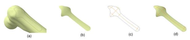
Figure 3: Select the region of interest and reconstruct it as the abutted surface of plate.
