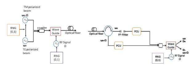
Figure 1. Transmitter and receiver to implement BB84 protocol. RNG=random number generator, FP=Fabry-Perot,  $D_0$  and  $D_1$  are single-photon detectors [10]. (©IEEE.)
