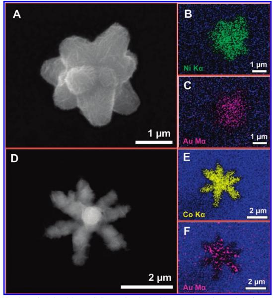
**Figure 3.** (A) SEM image of a single Au/Ni MF. (B,C) Corresponding Ni K $\alpha$ - and Au M $\alpha$ -based EDAX images collected from the sample shown in panel A. (D) Single particle SEM image of Au/Co MF. Co K $\alpha$ - and Au M $\alpha$ -based EDAX image of Au/Co MF (D) is shown in panels E and F, respectively. The amount of Ni and Co ions used during the synthesis was 0.3 mL (150 mM).
