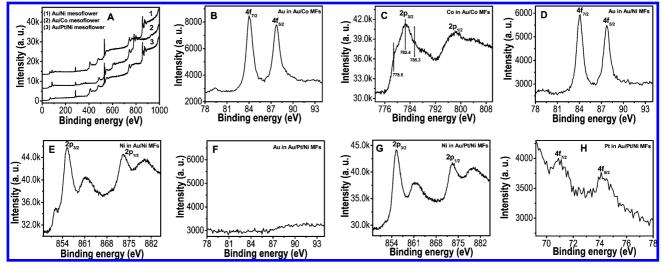
**Figure 7.** (A) Wide scan XPS spectra of Au/Ni, Au/Co, and Au/Pt/Ni MFs. (B,D,F) The Au 4f region of Au/Co, Au/Ni, and Au/Pt/Ni MFs, respectively. (C) XPS spectrum in the 2p region of Co in Au/Co MFs. (E,G) are the Ni 2p region of Au/Ni and Au/Pt/Ni MFs, respectively. (H) Pt 4f region of Au/Pt/Ni MFs.
