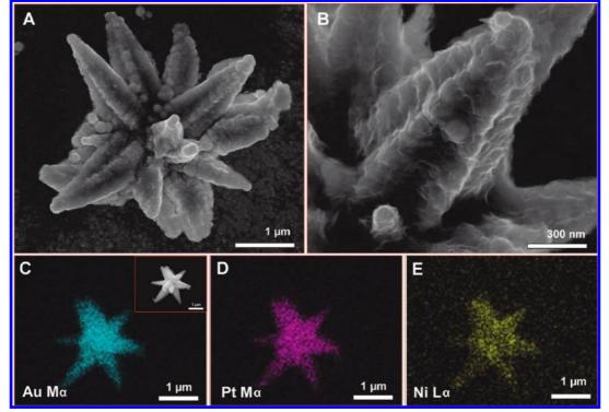
Figure 5. (A,B) The FESEM images of a single Au/Pt/Ni MF and an enlarged view of its stem, respectively. (C-E) The EDAX images of Au/Pt/Ni MF shown in the inset of panel C.
