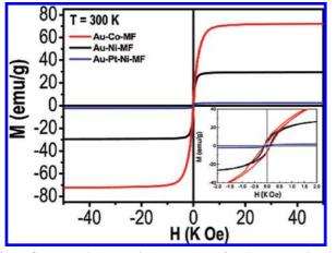
**Figure 8.** Magnetic hysteresis loops (M/H) of various magnetic MFs at 300 K. The inset shows the low-field part of the hysteresis loops. The amount of Ni and Co ions used during the synthesis was 0.3 mL (150 mM).
