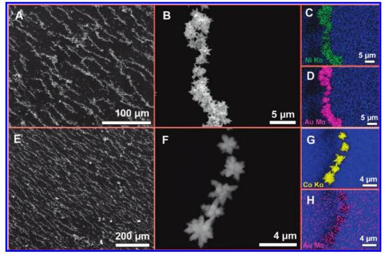
Figure 9. (A,E) SEM images showing the long-range, magnetic field-induced assembly of Au/Ni and Au/Co MFs, respectively. (B,F) Single strands of Au/Ni and Au/Co MF, respectively. Corresponding elemental maps are also given.
