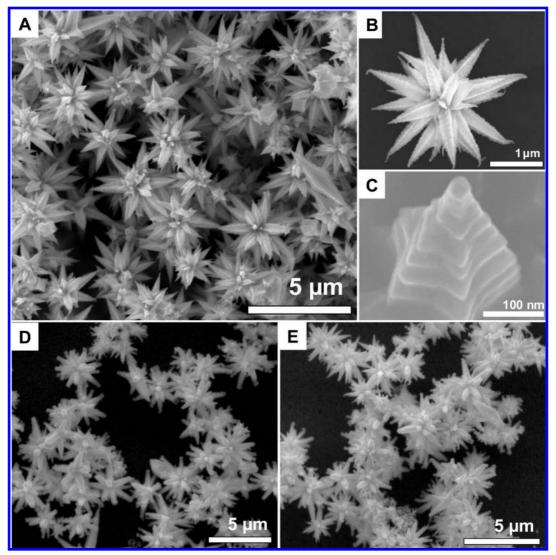
Figure 1. Large area SEM images of Au MFs (A) and a FESEM image of a single Au MF (B). The pentagonal symmetry of the stem is clearly visible in the top view of the stem shown in panel C. Large area SEM images of bimetallic Au/Ni (D) and Au/Co (E) MFs. In both cases, the amount of Ni and Co ions used during the synthesis was 0.1 mL (150 mM).
