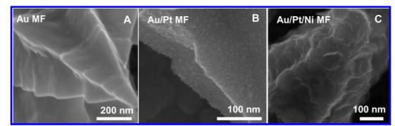
Figure 6. Magnified FESEM images of the stems of different MFs. (A) Au MF, (B) Au/Pt, and (C) Au/Pt/Ni MFs.
