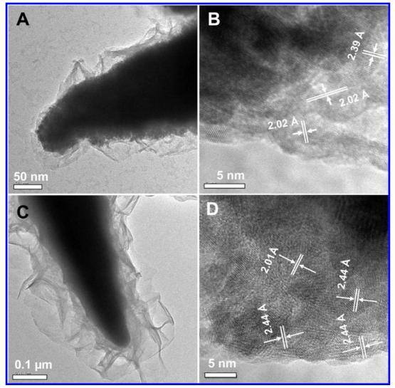
Figure 4. TEM images of the tip of the Au/Ni (A) and Au/Co (C) MFs. (B,D) Lattice-resolved images collected from the tip of the Au/Ni and Au/Co MFs, respectively. The amount of Ni and Co ions used during the synthesis was 0.1 (150 mM) and 0.3 mL (150 mM), respectively.
