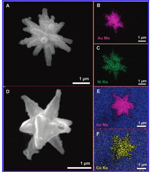
**Figure 2.** (A) SEM image of a single Au/Ni MF. (B,C) Corresponding Au M $\alpha$ - and Ni K $\alpha$ -based EDAX images collected from the sample shown in panel A. (D) Single particle SEM image of Au/Co MF. A Au M $\alpha$ - and Co K $\alpha$ -based EDAX image of Au/Co MF (D) is shown in panels E,F, respectively. The amount of Ni and Co ions used during the synthesis was 0.1 mL (150 mM).
