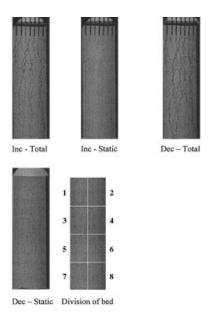
Figure 12. Liquid hysteresis X-ray images used to determine static and dynamic holdups quantitatively at 0.02 lpm liquid flow rate. Data are given in Table 3.
