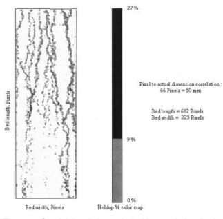
Figure 5. Spatial local dynamic holdup variation in the packed bed domain at 0.175 lpm.
