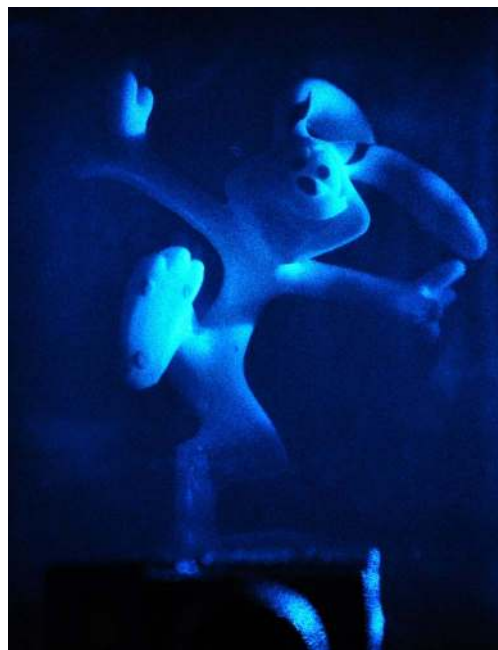
Fig. 10. (Color online) Hologram recorded using \text{Ar}^+ laser.
