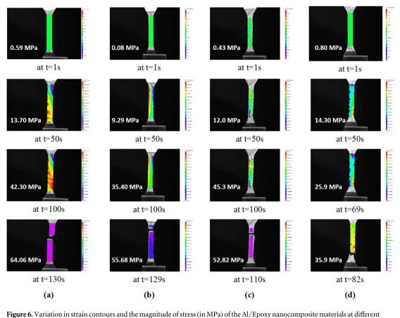
**Figure 6.** Variation in strain contours and the magnitude of stress (in MPa) of the Al/Epoxy nanocomposite materials at different instances during the tensile testing with the filler concentration (a) 0 wt%, (b) 1 wt%, (c) 5 wt% and (d) 10 wt%.
