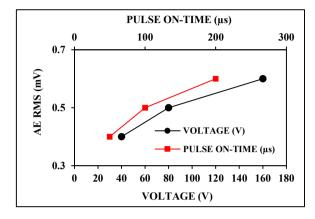
Fig. 6. (a) Comparison of AE RMS with voltage and pulse on-time
