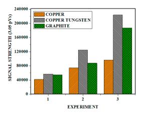
Fig. 5. (b) Signal strength comparison for copper, copper tungsten and graphite
