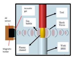
Fig. 2. Side view of the dielectric tank fitted with AE sensor
