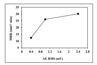
Fig. 7. (c) AE RMS vs. MRR
