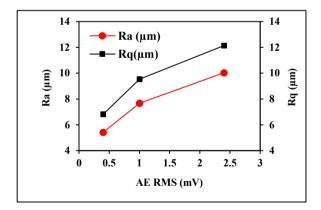
Fig. 7. (b) AE RMS vs. (Ra and Rq)
