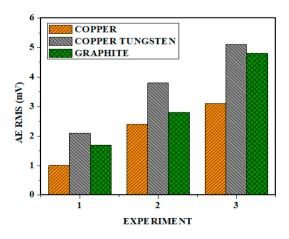
Fig. 5. (a) AE RMS comparison for copper, copper tungsten and graphite
