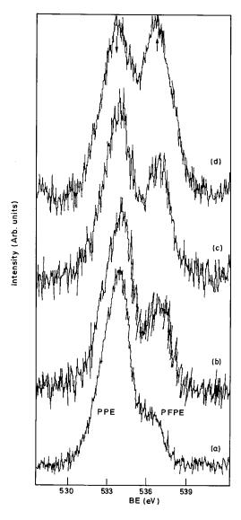
FIG. 2. X-ray photoelectron spectrum of the C 1s region of a mixture of perfluoropolyether and polyphenylether in the 1:100 volume ratio at various electron take-off angles. (a) 80, (b) 50, (c) 30, (d)  $10^0$ . Arrows indicate the direction of intensity variation.
