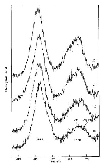
FIG. 1. X-ray photoelectron spectrum of the C 1s region of a mixture of perfluoropolyether and polyphenylether in the 1:100 volume ratio at various electron take-off angles. The various features are indicated. (a) 80, (b) 50, (c) 30, (d) 10<sup>0</sup>. Note the increase in intensity of the CF<sub>2</sub>/CF<sub>3</sub> feature as the take-off angle is decreased. Arrows show the direction of intensity variation.
