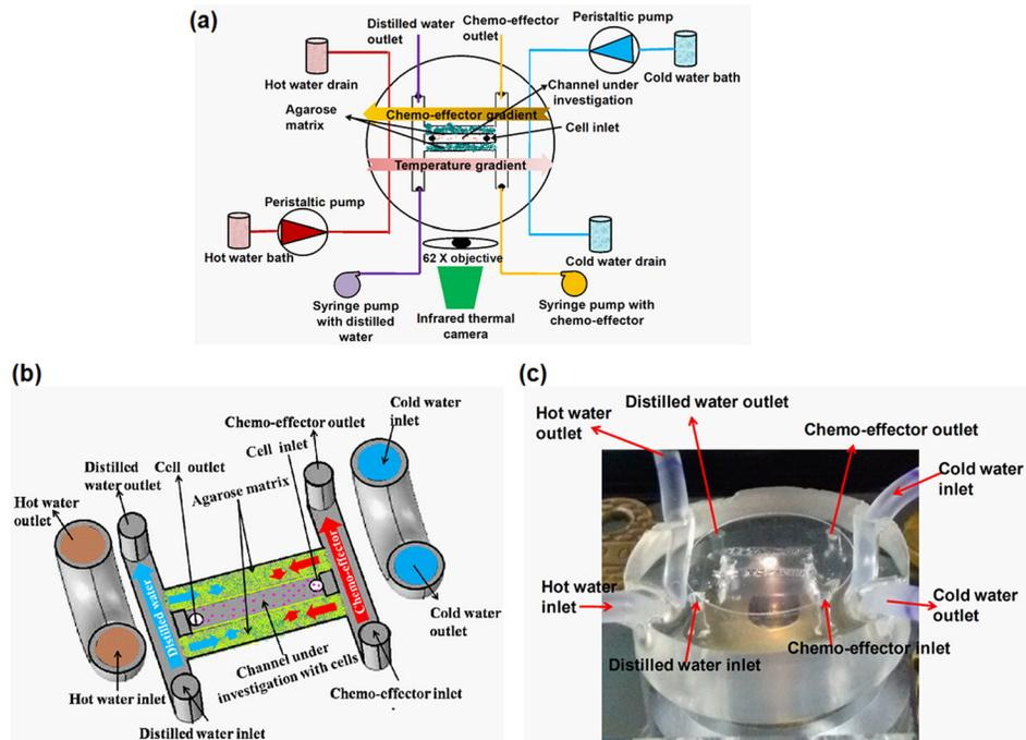
FIG. 1. (a) Sketch of the experimental setup for the cell migration study under imposed competing chemical and thermal gradients. (b) Schematic illustration of the channels in the device. (c) Schematic view of the microfluidic device under working conditions.
