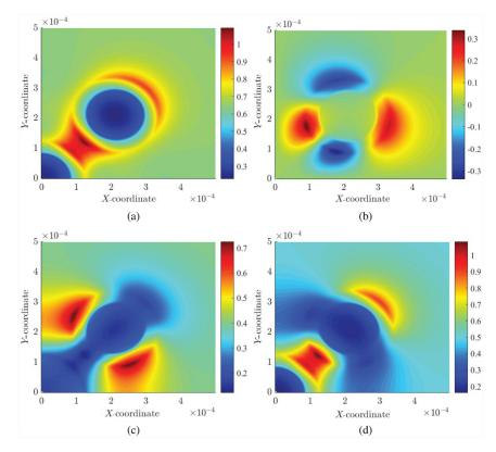
Figure 13. Case 2 for generalized Gent model. (a) ||T|| (b) Shear stress component,  $T_{r\theta}$ . (c) Radial stress. (d) Circumferential stress.
