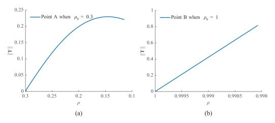
Figure 5. Variation of norm of the stress tensor with density for the generalized Gent model (case 2). (a) At point A. (b) At point B.
