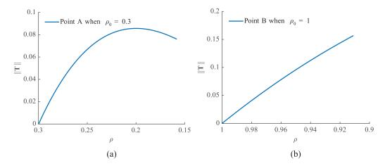
Figure 9. Variation of the norm of the stress tensor with density for generalized neo-Hookean model (case 2). (a) At point A. (b) At point B.
