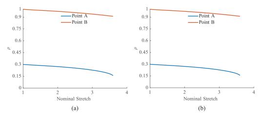
Figure 7. Density variation with nominal stretch for the generalized neo-Hookean model. (a) Case I. (b) Case 2.
