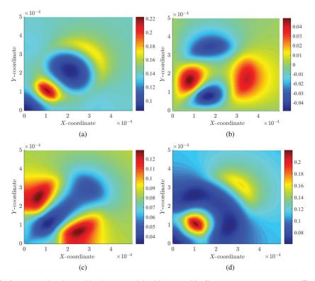
Figure 11. Case 2 for generalized neo-Hookean model. (a) ||T|| (b) Shear stress component,  $T_{r\theta}$ . (c) Radial stress. (d) Circumferential stress.
