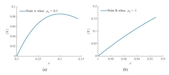
Figure 8. Variation of the norm of the stress tensor with density for generalized neo-Hookean model (case 1). (a) At point A. (b) At point B.
