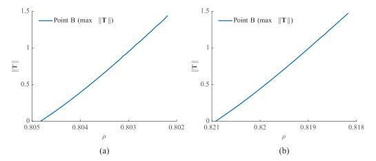
Figure 6. Variation of the maximum of the norm of the stress tensor with density for the generalized Gent model. (a) Case 1. (b) Case 2.
