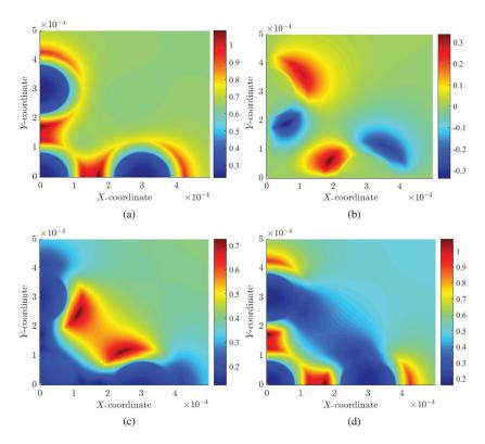
Figure 12. Case I for generalized Gent model. (a) ||T|| (b) Shear stress component. (c) Radial stress. (d) Circumferential stress.
