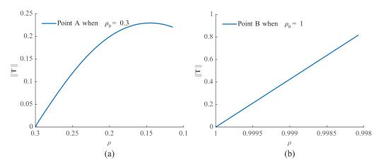
Figure 4. Variation of the norm of the stress tensor with density for the generalized Gent model (case 1). (a) At point A. (b) At point B.
