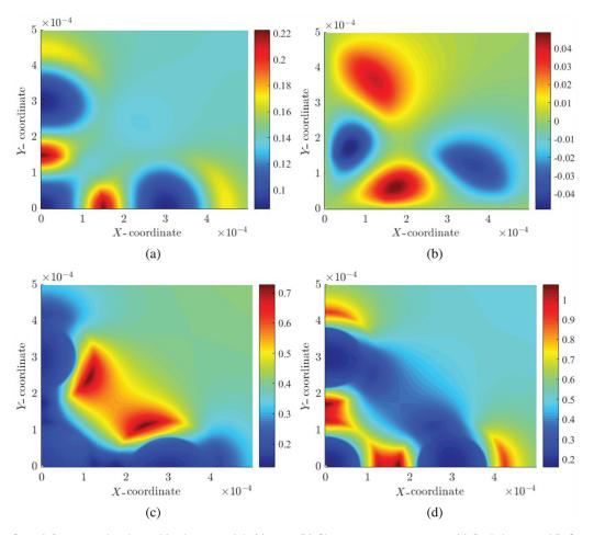
Figure 10. Case I for generalized neo-Hookean model. (a) ||T|| (b) Shear stress component. (c) Radial stress. (d) Circumferential stress.
