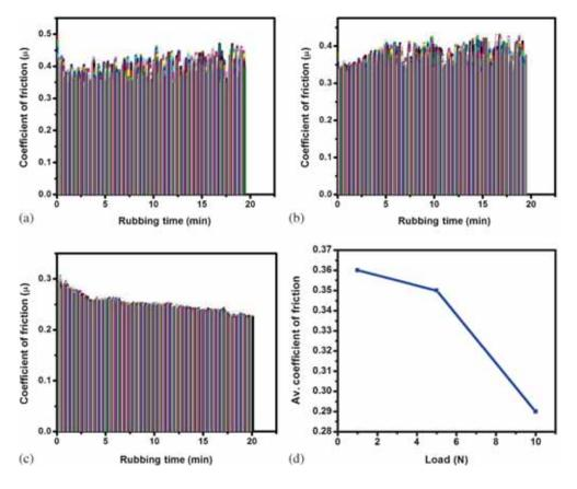
Figure 5. Variation of friction coefficient of undoped multilayer-diamond coatings, sliding against  $Al_2O_3$  ball with respect to (a) normal load and duration of rubbing at (a) 1, (b) 5 and (c) 10 N loads. (d) Average coefficient of friction and normal load.
