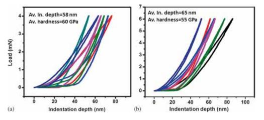
Figure 4. Load-displacement curves corresponding to six indentations on multilayer CVD-diamond coatings: (a) undoped and (b) boron-doped.
