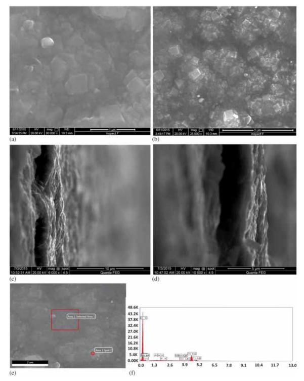
**Figure 3.** Surface morphologies of (a) undoped coatings and (b) boron-doped diamond coatings. Cross-sectional images of (c) undoped coating and (d) boron-doped diamond coating. (e, f) Energy dispersive X-ray analysis (EDXA) of undoped diamond coatings. (g) Element wise compositions and % atomic weight of undoped multilayer CVD-diamond coating system. (h) EDXA of boron-doped diamond coatings. (i) element wise composition and % atomic weight of boron-doped multilayer CVD-diamond coating system.
