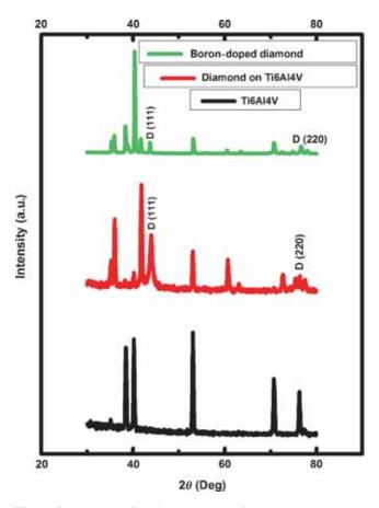
**Figure 2.** X-ray diffraction patterns of uncoated, multilayer CVD-diamond coatings and boron-doped diamond coatings.
