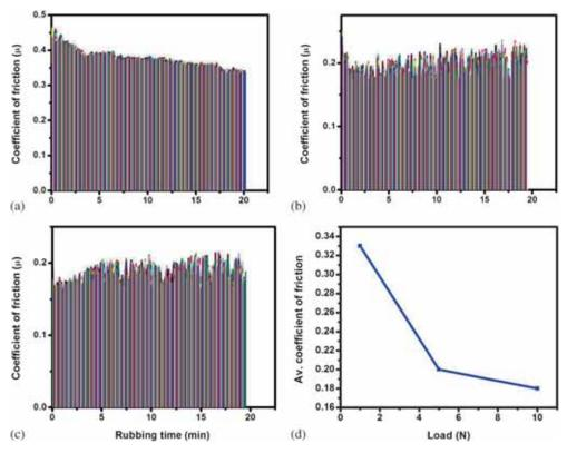
**Figure 6.** Variation of friction coefficient of doped multilayer-diamond coatings, sliding against  $Al_2O_3$  ball with respect to normal load and duration of rubbing at (**a**) 1, (**b**) 5 and (**c**) 10 N loads. (**d**) Average coefficient of friction and normal load.
