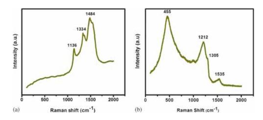
Figure 1. Raman spectra of multilayer CVD-diamond coatings: (a) undoped and (b) boron doped.
