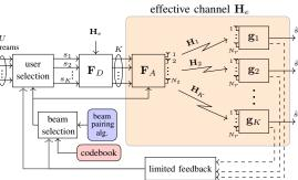
[6],  $\mathbf{H}_e$  should be known at the transmitter. User k needs to feedback the  $k^{th}$  row of the effective channel  $\mathbf{H}_e$  given by
