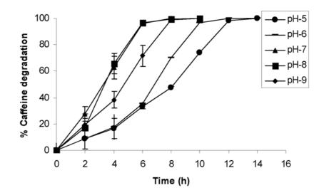
**Fig. 2** Effect of pH on caffeine degradation by induced cells of *Pseudomonas sp.* All experiments were performed in triplicate. The initial concentration of caffeine and induced cells was at 1.2 g/l and 8 g/l, respectively. The temperature and agitation rate was maintained at 30°C and 180 rpm respectively.
