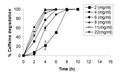
**Fig. 1** Effect of cell concentration on caffeine degradation by induced cells of *Pseudomonas sp.* All experiments were performed in triplicate. The initial concentration of caffeine was at 1.2 g/l. The initial pH, temperature and agitation rate was maintained at 7.0, 30°C and 180 rpm respectively.
