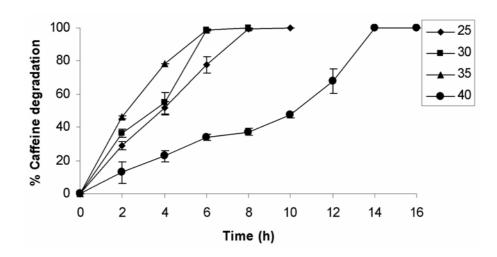
**Fig. 3** Effect of temperature on caffeine degradation by induced cells of *Pseudomonas sp.* All experiments were performed in triplicate. The initial concentration of caffeine and induced cells was at 1.2 g/l and 8 g/l, respectively. The initial pH and agitation was maintained at 7.0 and 180 rpm.
