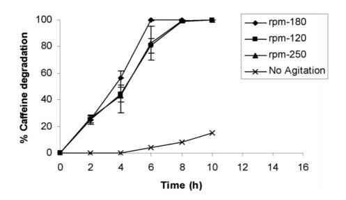
**Fig. 4** Effect of agitation on caffeine degradation by induced cells of *Pseudomonas sp.* All experiments were performed in triplicate. The initial concentration of caffeine and induced cells was at 1.2 g/l and 8 g/l, respectively. The initial pH was maintained at 7.0 and the temperature was maintained at 35°C.
