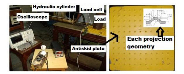
Figure 1. Experimental setup for friction test
