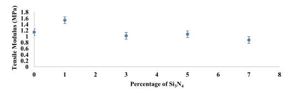
Figure 5. Tensile modulus of NR/SBR compounds with and without Si<sub>3</sub>N<sub>4</sub> at 100% elongation
