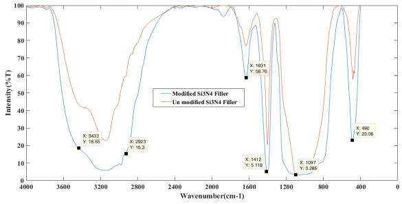
Figure 3. FTIR spectra of modified Si<sub>3</sub>N<sub>4</sub>and unmodified Si<sub>3</sub>N<sub>4</sub>
