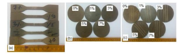
Figure 2. (a) Tensile test Specimens (b) Specimens-before friction testing (c) Friction tested specimens
