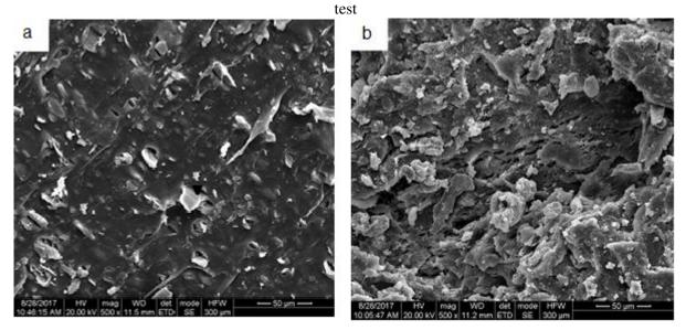
Figure 9. SEM micrograph of rubber specimen with 1% filler (b) before friction test (b) after friction test
