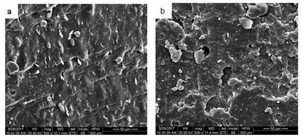
Figure 8. SEM micrograph of rubber specimen without filler (b) before friction test (b) after friction
