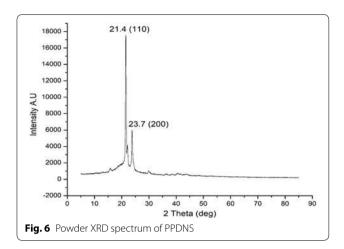
various samples irrespective of their physical state. The powder XRD pattern of PPDNS is shown in Fig. 6. The spectrum indicates that the semi-crystalline lattice structure of the drug-incorporated nanospheres with peak intensities corresponding to PEG polymer. However, the nanospheres appear in powder state due to the blend of PCL/PEG. The diffraction pattern is characteristic of the PPDNS sample.
