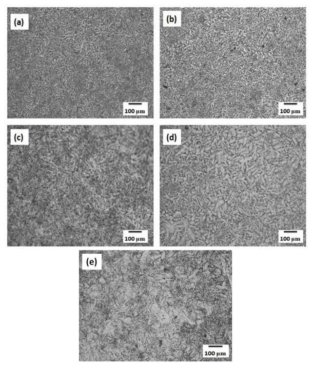
Figure 6. Micrographs of (a) NTCu2, (b) NTCu4, (c) NTCu6, (d) NTCu8 and (e) NTCu10 alloys.
