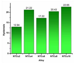
Figure 4. Thermal Hysteresis of the alloys studied.
