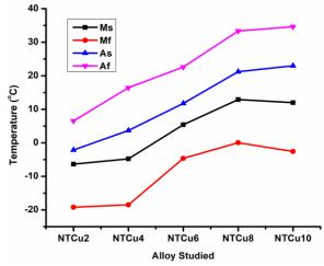
Figure 3. Variation of transformation temperatures with copper content.
