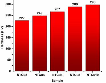
Figure 5. Hardness measurements of different NiTiCu SMAs.
