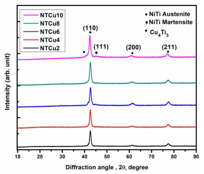
Figure 1. XRD results of NiTiCu alloys.
