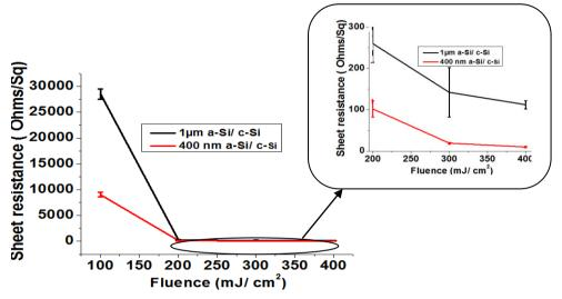
Figure 7. Resistance of ns- laser treated samples at the wavelength of 355 nm treated with different fluences with 30 % of spot overlap in air.
