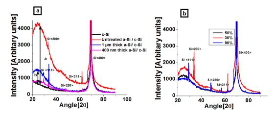
Figure 6. (a) XRD data of the untreated and laser treated a-Si/c-Si sample for the laser fluence of 200 mJ/cm<sup>2</sup> and Gaussian beam profile with 50% spot overlap (b) different percentages of spot overlap with 400 mJ/cm<sup>2</sup>.
