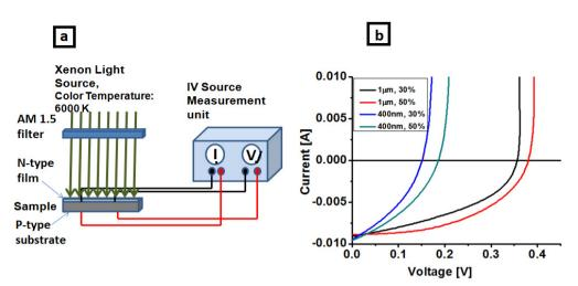
**Figure 8.** (a) IV measurement setup and (b) IV characteristics of laser treated PN photovoltaic cell under illumination with Gaussian beam profile in air with  $200 \text{mJ/cm}^2$ .
