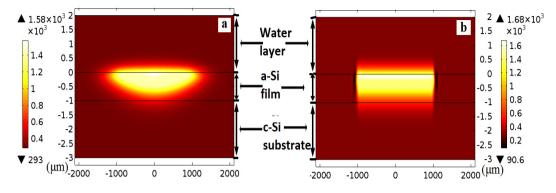
**Figure.10** Temperature distribution profile in two dimensional for (a) Gaussian beam and (b) flat-top beam for  $400 \text{ mJ/cm}^2$ .
