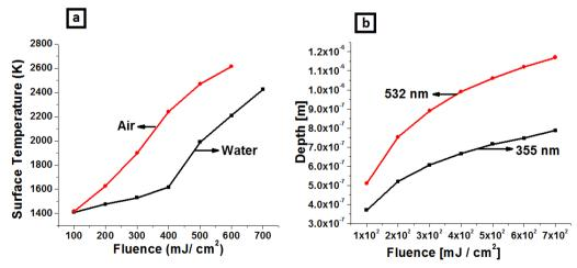
**Figure 11.** (a) Temperature rise during laser irradiance at the surface for different laser fluence in air and water (b) Depth of crystallization with different fluence values with 532 nm and 355nm.
