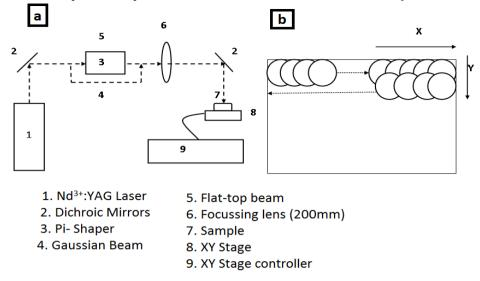
**Figure 1.** (a) Experimental setup for nanosecond Laser annealing with Flat-top and Gaussian beams (b) Laser annealing and texturing with spot overlap.
