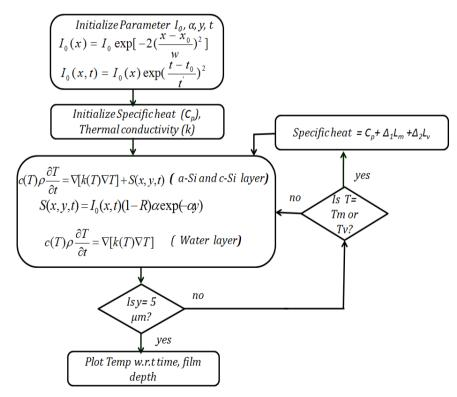
Figure 9. Flow chart for the numerical analysis with heat transfer equation.
