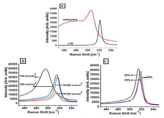
Figure 5. Raman spectroscopy of the (a) untreated and laser treated a-Si/c-Si samples in air at 355 nm with (b) with different fluence values for 50% spot overlap with Gaussian beam (c) different percentage of spot overlap with  $400 \text{mJ/cm}^2$ .
