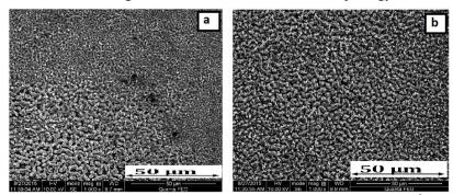
**Figure 4.** SEM images of a-Si / c-Si samples irradiated with 20 pulses of fluence  $200 \text{mJ/cm}^2$  in air with (a) Gaussian and (b) flat-top beam profiles (Images with 1000X magnification).
