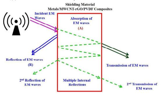
Scheme 2. Schematic representation of EMI Shielding Material
