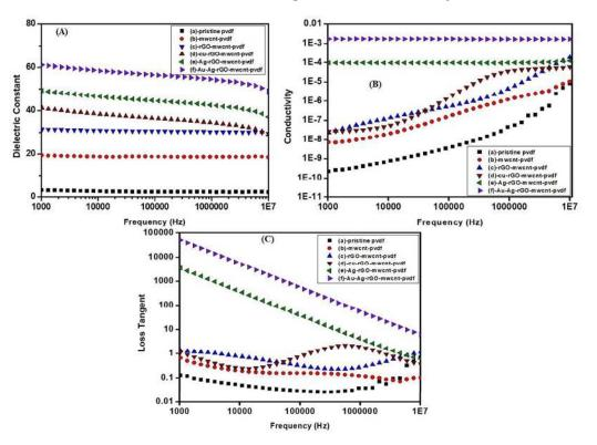
Fig 5A. Dielectric Constant (a), Electrical Conductivities(b), Dielectric Loss(c) of Pristine PVDF(A), MWCNT-PVDF(B), rGO-MWCNT-PVDF(C), Cu-rGO-MWCNT-PVDF(D) composites
