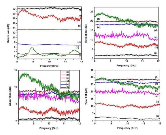
Fig 6A. Return loss, Reflection, Absorption and Effective EMI SE(d) at 12 GHz respectively for (a) Pristine PVDF, (b) MWCNT-PVDF, (c) rGO-MWCNT-PVDF,(d)Cu-rGO-MWCNT-PVDF composites
