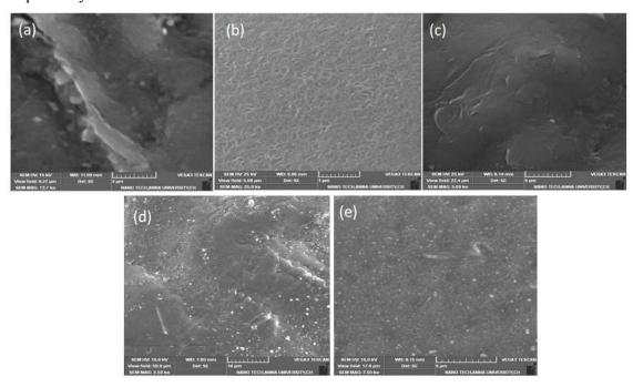
Fig 2. SEM Micrographs for Pristine PVDF (a), MWCNT-PVDF (b), rGO-MWCNTPVDF (c), Cu decorated rGO-MWCNT-PVDF (d) and Ag-Au decorated rGO-MWCNT-PVDF (e) Composites
