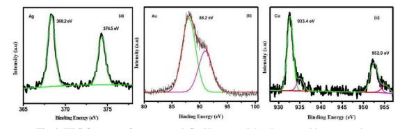
Fig 4. XPS Spectra of Ag, Au and Cu Nanoparticles decorated in composites
