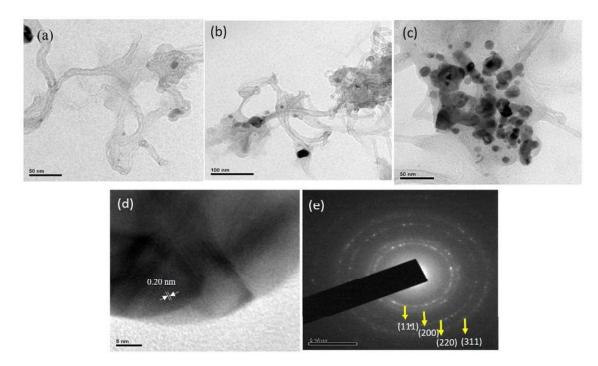
Fig 3. HRTEM image of rGO-MWCNT (a), Cu decorated rGO-MWCNT (b), Ag-Au decorated rGO-MWCNT (c), high resolution image (d) and its SAED patterns (e X-ray Photoelectron Spectra (XPS) Analysis
