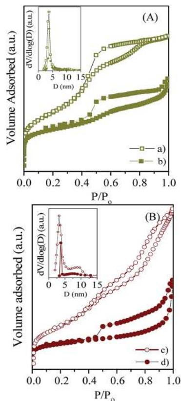
Fig. 3 N<sub>2</sub> adsorption–desorption isotherms of pristine OMC (A) and nitrogenous carbon (B): (a) CSI-809, (b) LFP/CSI-809, (c) MNC-859, and (d) LFP/MNC-859.
