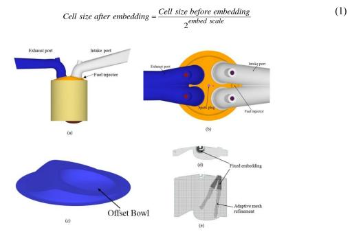
**Figure 2.** (a) Computational domain of the engine (b) Top view of engine (c) Piston with offset piston (d) Embedding at Spark (e) Adaptive mesh refinement at fuel injection
