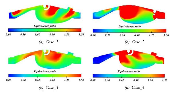
Figure 6. Comparison of ER distribution on the central plane at the spark timing
