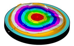
**Figure 7.** Hemispherical zones in the combustion chamber with spark plug as centre
