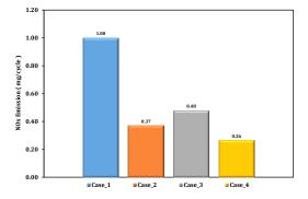
**Figure 14.** Comparison of NOx emission at EVO for various cases of SP and FI location
