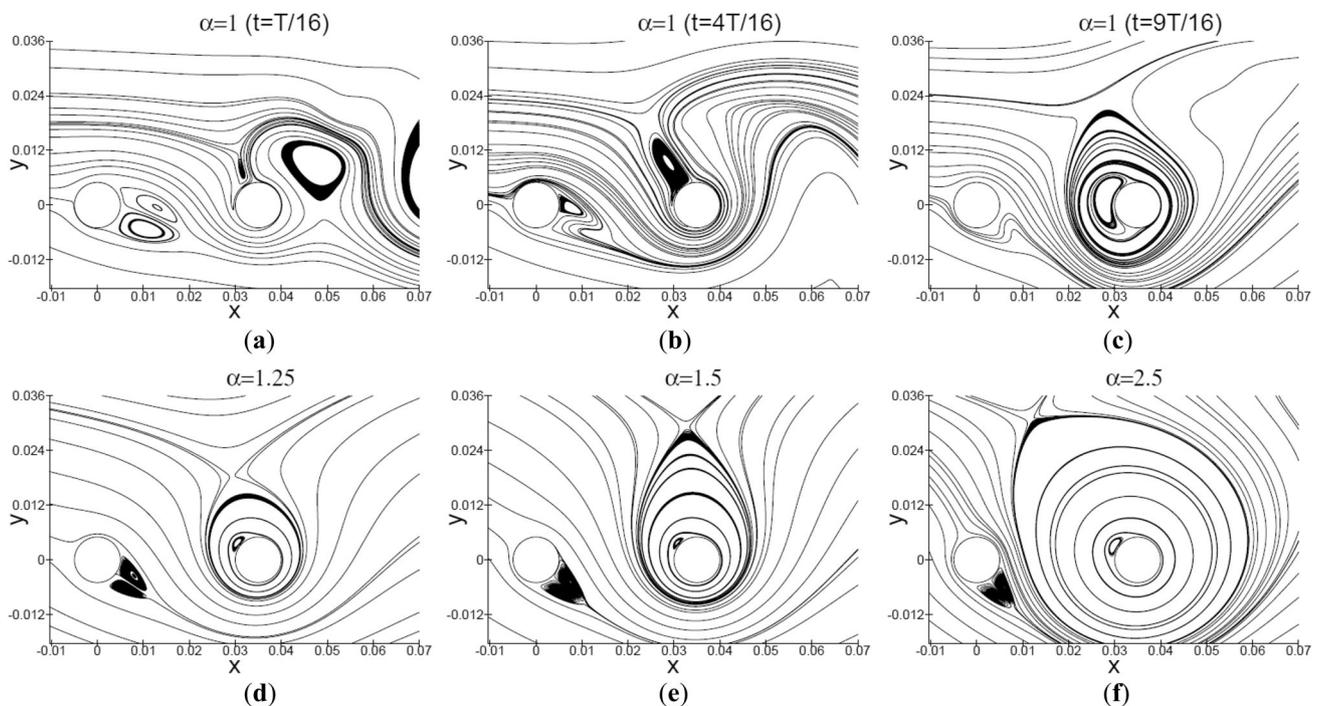
**Figure 9.** Streamline plots for  $s = 3.5d$  (a)  $\alpha = 1$  and  $t = T/16$ , (b)  $\alpha = 1$  and  $t = T/4$ , (c)  $\alpha = 1$  and  $t = 3T/4$ ; steady streamlines for (d)  $\alpha = 1.25$ , (e)  $\alpha = 1.5$ , (f)  $\alpha = 2.5$ .
