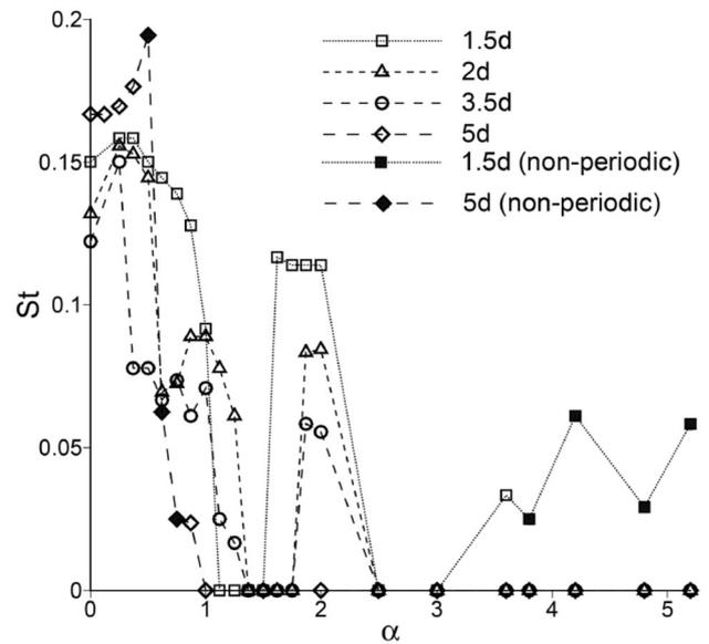
**Figure 14.** Variation of Strouhal number ( $St$ ) with  $\alpha$  for different values of inter-cylinder spacing (the darkened scatters correspond to non-periodic flow).
