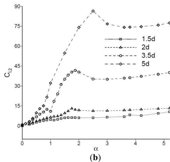
**Figure 13.** Variation of RMS lift coefficient with rotational speed for different values of inter-cylinder spacing on (a) upstream cylinder and (b) downstream cylinder.
