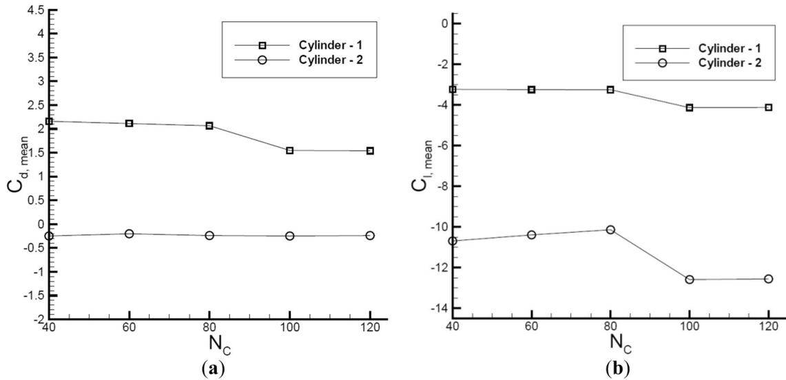
Figure 3. Variation of  $C_l$  and  $C_d$  for different grids for  $s = 2d$  and  $\alpha = 3$ .
