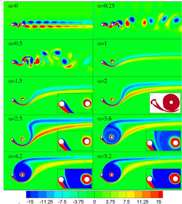
**Figure 8.** Instantaneous vorticity contours for different values of  $\alpha$  and  $s = 5d$ .
