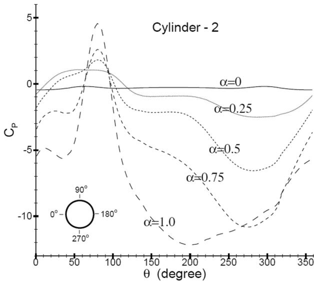
**Figure 12.** Time-averaged distribution of pressure coefficient on the surface of downstream cylinder at low rotational speeds ( $\alpha < 1$ ), for  $s = 3.5d$ .
