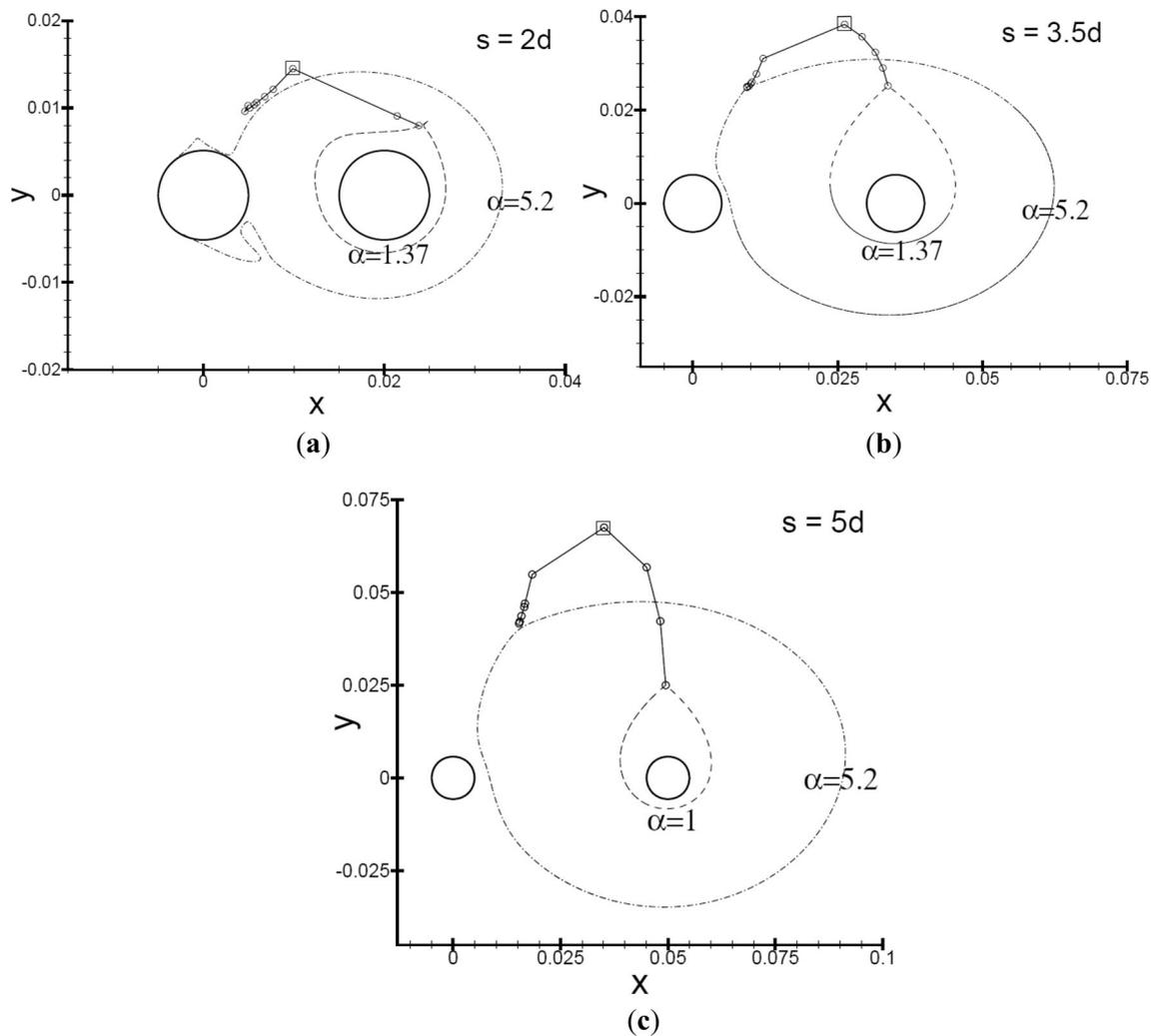
**Figure 10.** Locations of stagnation points with increase in rotational speed for inter-cylinder spacing values of (a) 2d, (b) 3.5d and (c) 5d.
