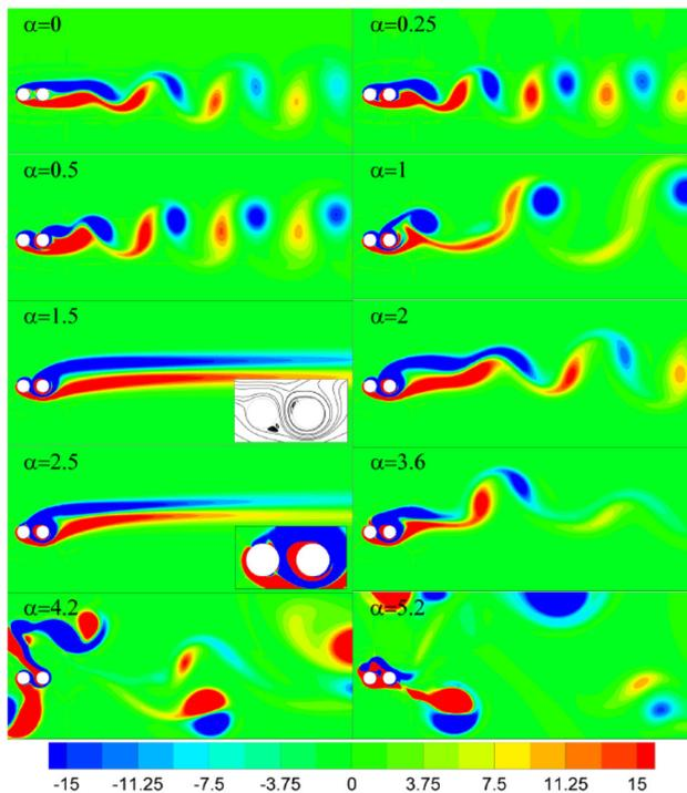
**Figure 6.** Instantaneous vorticity contours for different values of  $\alpha$  and  $s = 1.5d$ .
