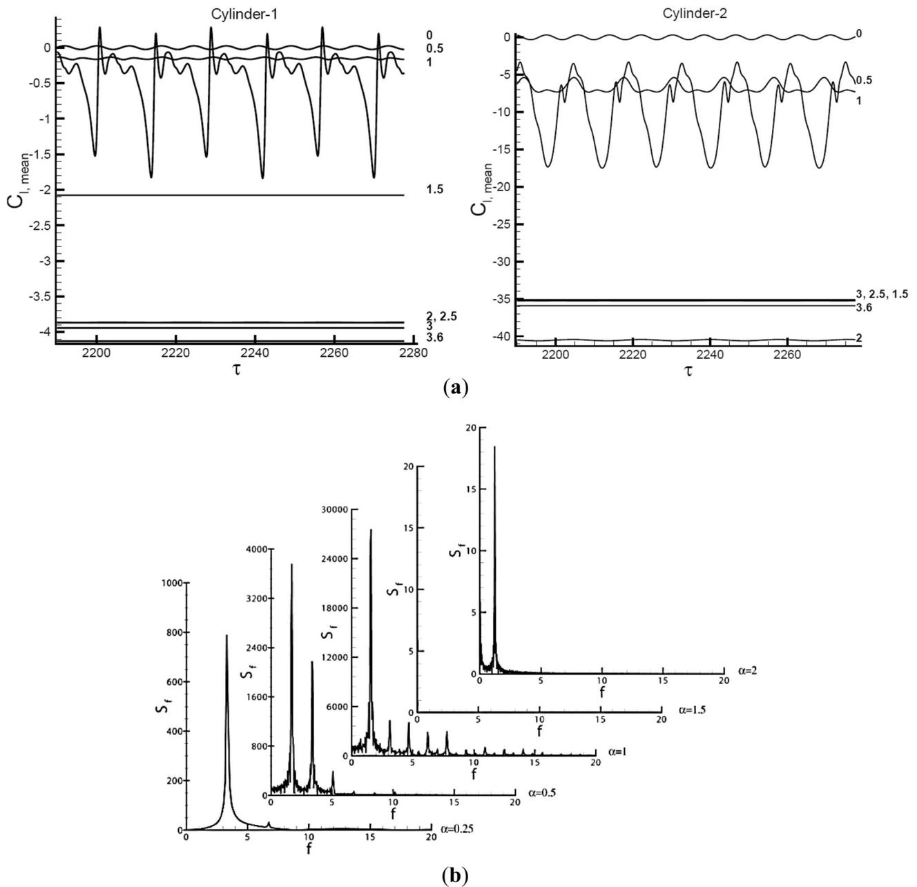
**Figure 15.** (a) Variation of lift on both the cylinders and (b) spectra of the lift signal of downstream cylinder, for  $s = 3.5d$ .
