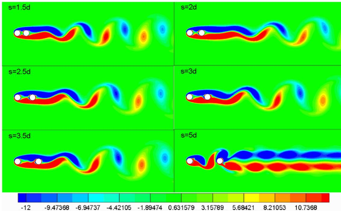
Figure 5. Instantaneous vorticity contours for different values of  $s$  at  $\alpha = 0$ .
