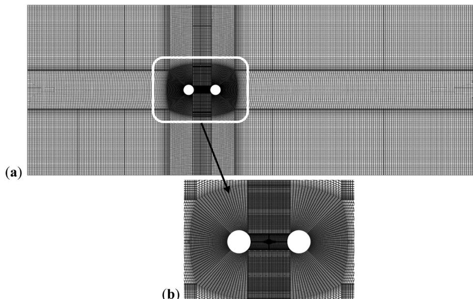
**Figure 2.** (a) Schematic of grid mesh in whole domain, (b) magnified view of mesh close to cylinder.
