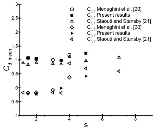
Figure 4. Variation of mean drag coefficient with inter-cylinder spacing for flow past two stationary circular cylinders in tandem.
