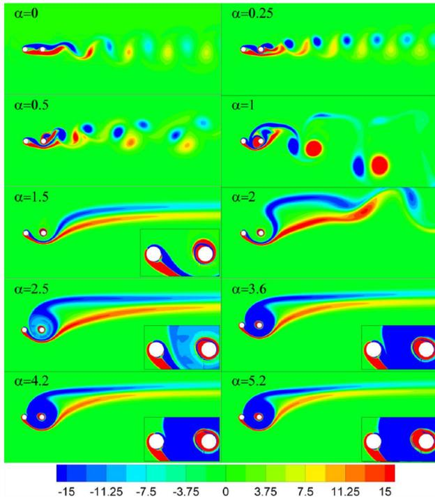
**Figure 7.** Instantaneous vorticity contours for different values of  $\alpha$  and  $s = 3.5d$ .
