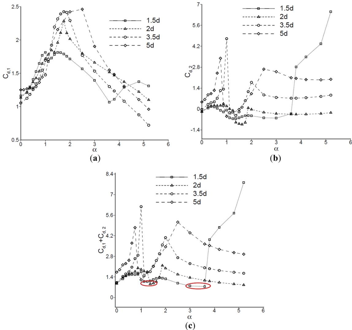
**Figure 11.** Variation of mean drag coefficient with rotational speed for different values of  $s$ , for (a) upstream cylinder, (b) downstream cylinder and (c) both cylinders.
