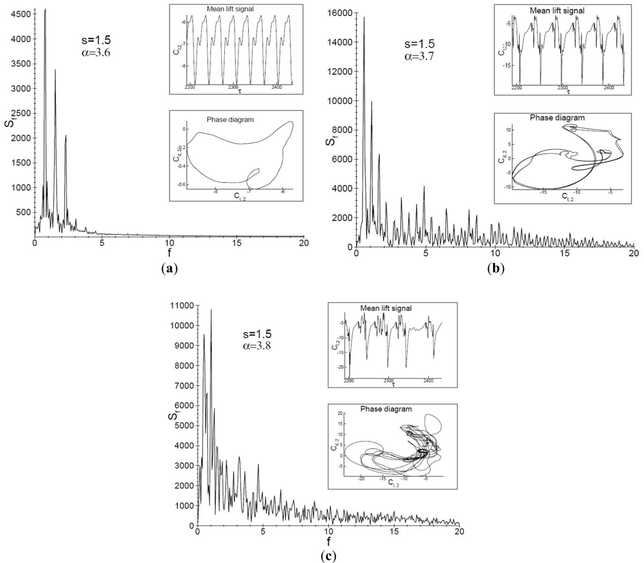
**Figure 16.** Temporal characterization of downstream cylinder wake for  $s = 1.5d$  (a)  $\alpha = 3.6$ , (b)  $\alpha = 3.7$  and (c)  $\alpha = 3.8$ .
