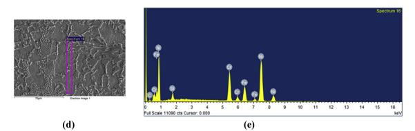
Fig. 5. (a) Supra 55-Scanning Electron Microscope with EDS attachment. Fig. 5(b) and (c) Micrograph and EDS results at a height of 500  $\mu$ m above the interface of grooved specimen. Fig. 5 (d) and (e) Micrograph and EDS results at a height of 500  $\mu$ m above the interface of un-grooved specimen.
