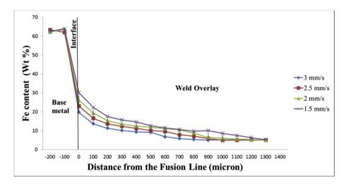
Fig. 7. Variation in Fe content of grooved specimens over the hardness-affected region.
