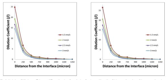
Fig. 8. Variation of Dilution coefficients at different locations from the interface into weld overlay of (a) grooved specimen (b) un-grooved specimen.
