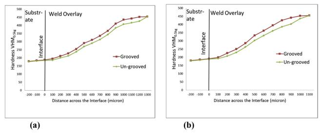
Fig. 6. Hardness distribution across the interface in the diluted region of the weld overlay for the travel speed of (a) 2 mm/s (b) 3 mm/s.
