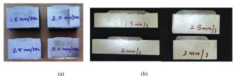
Fig. 2. Cut-sections of defect-free (a) Grooved specimens as deposited (b) Un-grooved specimens as machined.
