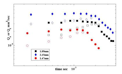
Fig 6: variation of the measured filling rate of cavity with time, for bubbles in water. Open markers represent the radial discharge  $Q_s$  and the filled markers represent the total discharge  $Q_t$ .
