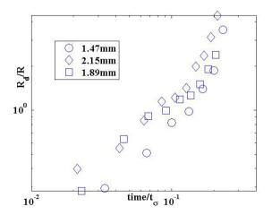
Fig 7: Variation of dimensionless cavity curvature (R<sub>d</sub>) against dimensionless time, measured for bubbles in water.
