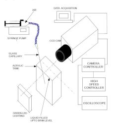
Fig 1: Schematic of the experimental set up
