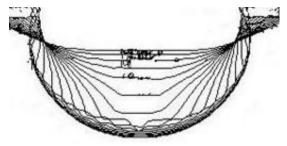
Fig 5: Superimposed contours of cavity collapse for R=2.15mm in water. Contours are separated by 0.25 milli seconds.
