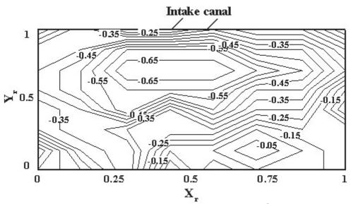
FIGURE 4. Contour map of bed after experiment with 8-2-15<sup>0</sup> arrangement
