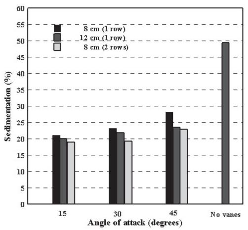
FIGURE 3. The variation of sedimentation (%) for different arrangement
