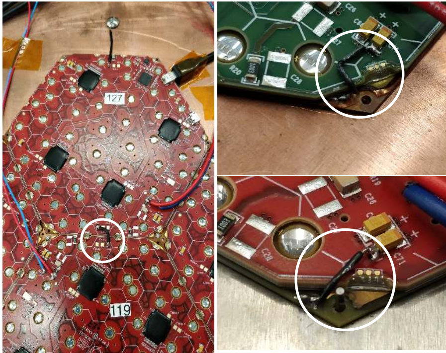
Figure 19: An example layer of the silicon CE-H with the ground connection between its central module and a peripheral module (left). An example of the ground connection for a double-Kapton™ module (top right). An example of the ground connection for a PCB baseplate module (bottom right).
