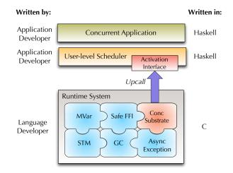
Figure 2. New GHC RTS design with Concurrency Substrate.
