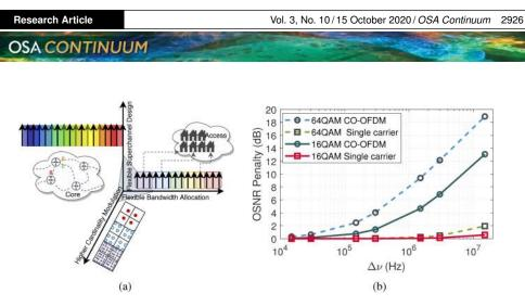
**Fig. 1.** (a) Multi-dimensional agility of coherent optical OFDM (b) OSNR penalty evaluated for a BER of  $1 \times 10^{-3}$  at various linewidth for systems employing 16/64QAM CO-OFDM and Nyquist shaped single carrier modulation with baseband sampling rate/symbol rate of 30 GS/s.
