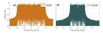
**Fig. 6.** Baseband spectrum of the generated (a) 16QAM CO-OFDM signal (19 GHz bandwidth) and (b) 64QAM CO-OFDM signal (10 GHz bandwidth).
