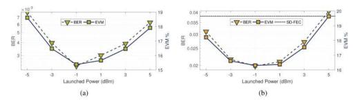
**Fig. 8.** Launched power optimization performed for 8 channel 16QAM CO-OFDM transmission showing BER and EVM vs launched power (b) Launched power optimization performed for 8 channel 32QAM CO-OFDM transmission showing BER and EVM vs launched power.
