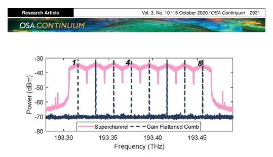
Fig. 7. Spectrum of the 8 channel 608 Gbps 16QAM CO-OFDM superchannel.
