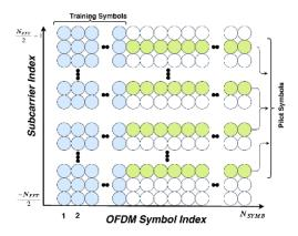
**Fig. 5.** Time and frequency distribution of OFDM symbols including the training symbols and pilot symbols.
