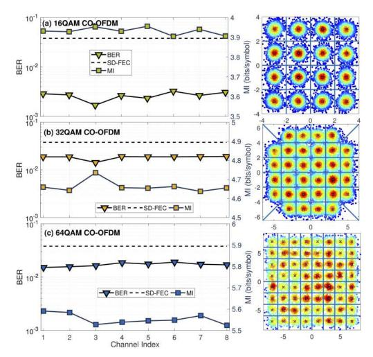
**Fig. 9.** BER performance and corresponding constellation diagram (CH4 data) of (a) 608 Gbps 16QAM CO-OFDM data (b) 760 Gbps 32QAM CO-OFDM data and (c) 480 Gbps 64QAM data at every channel of the three superchannel configurations.
