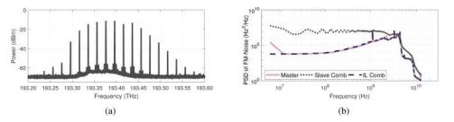
**Fig. 3.** (a) Output spectrum of the injection locked gain-switched comb (b) FM-noise spectrum of the master laser and that of a comb line before and after the injection.
